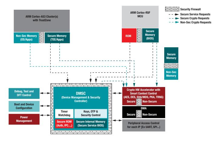
Figure 9. DMSC features in the Sitara AM65xx processor
