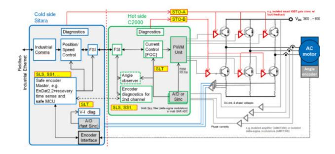
Figure 10. Example of safe implementation of Servo Drive
