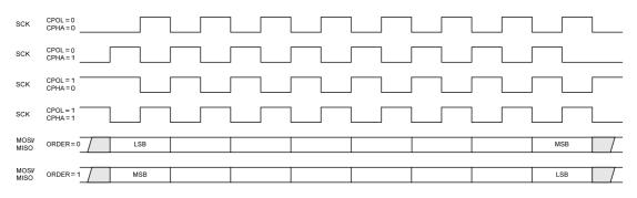
Figure 1. Phase, Polarity, and Bit Order
