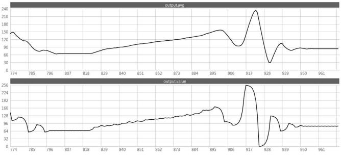
Figure 5. Voltage Follower Output With (Top) and Without (Bottom) 8-Value Averaging
