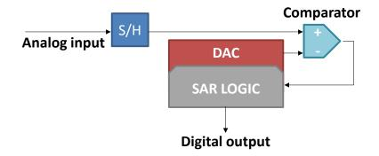
Figure 1. SAR ADC Block Diagram
