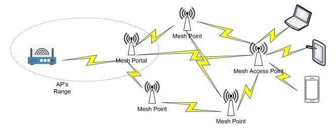
Figure 1-2. Wi-Fi Mesh Network Topology
