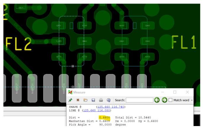
Figure 1-6. Via Placement and Distance between CC1352P / CC2652P and the PA IPC (FL2)
