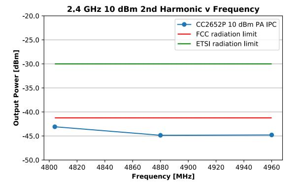
Figure 2-2. CC2652P - 2nd Harmonic versus Frequency
