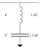
Figure 3-1. Circuit Diagram of the Notch Filter.
