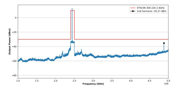
Figure 3-2. 2.4-GHz ETSI EN300 220 Radiated Emissions at 10-dBm Output
