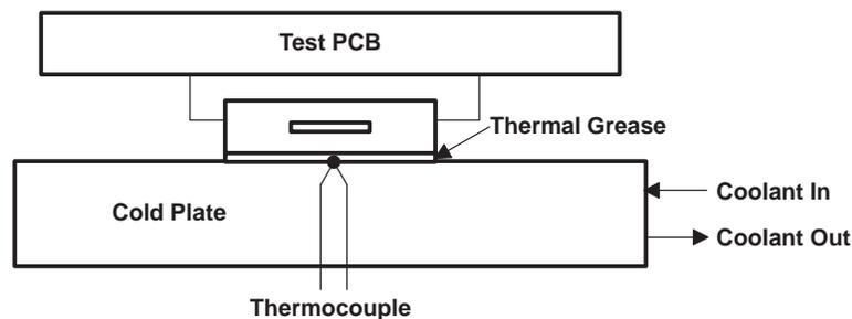
**Figure 2.  $\theta_{JC}$  Laboratory Measurement Method**
