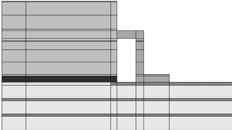
**Figure 4. Cross Section of 20-Pin SOIC Package on 2s2p PCB**
