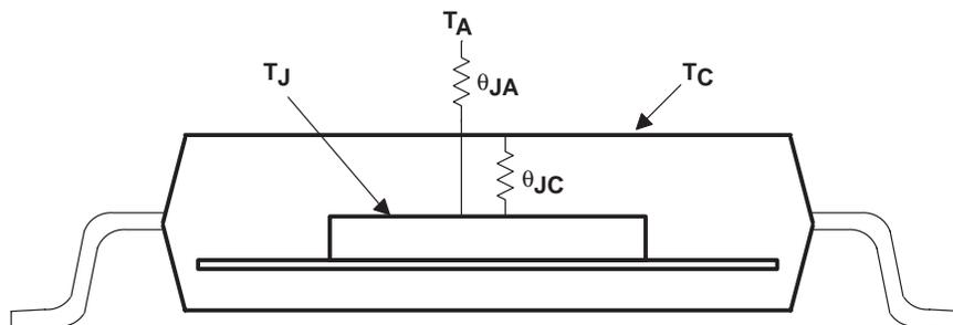
Figure 1. IC Package Thermal Metrics
