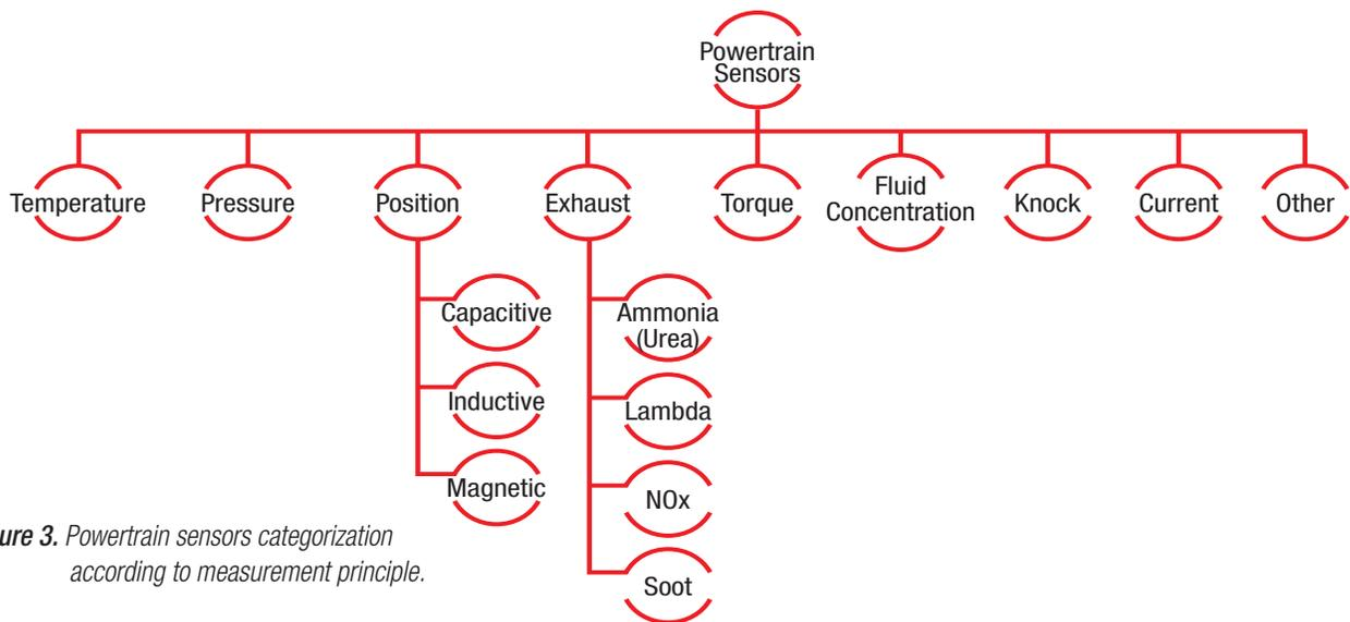
**Figure 3.** Powertrain sensors categorization according to measurement principle.
