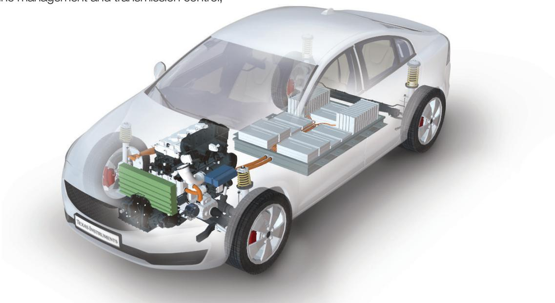
*Figure 1. The powertrain system in an HEV.*
