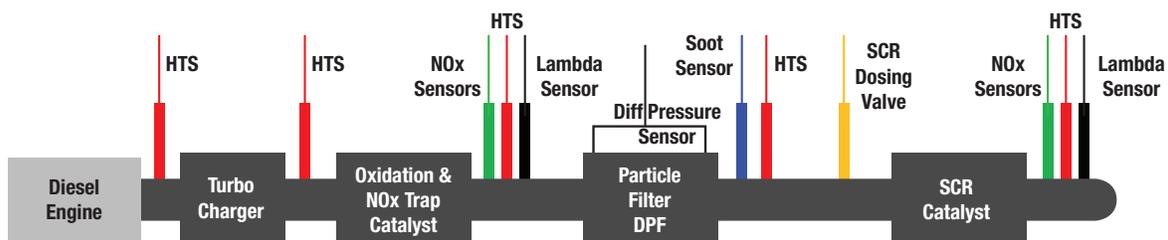
**Figure 4.** Types of sensors in an automotive exhaust system.
