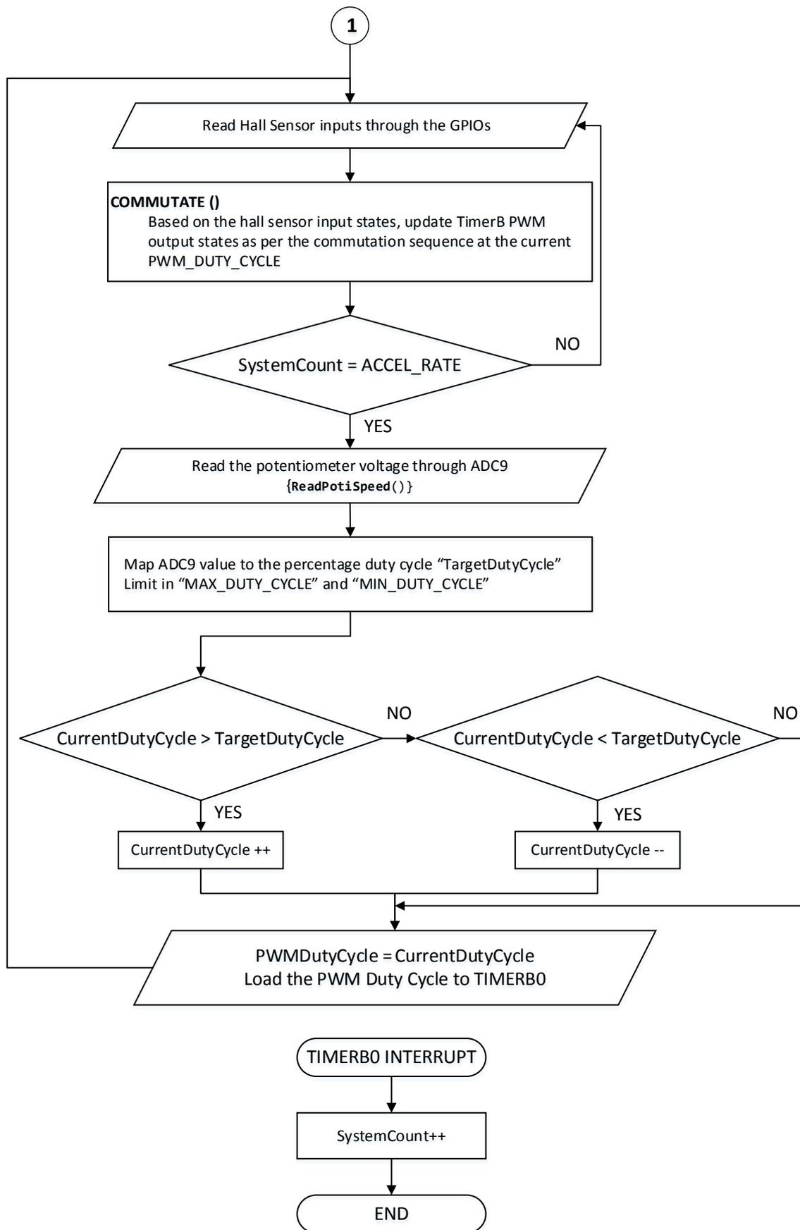
Figure 7. Flowchart of Sensor-Based Control Using DRV92250
