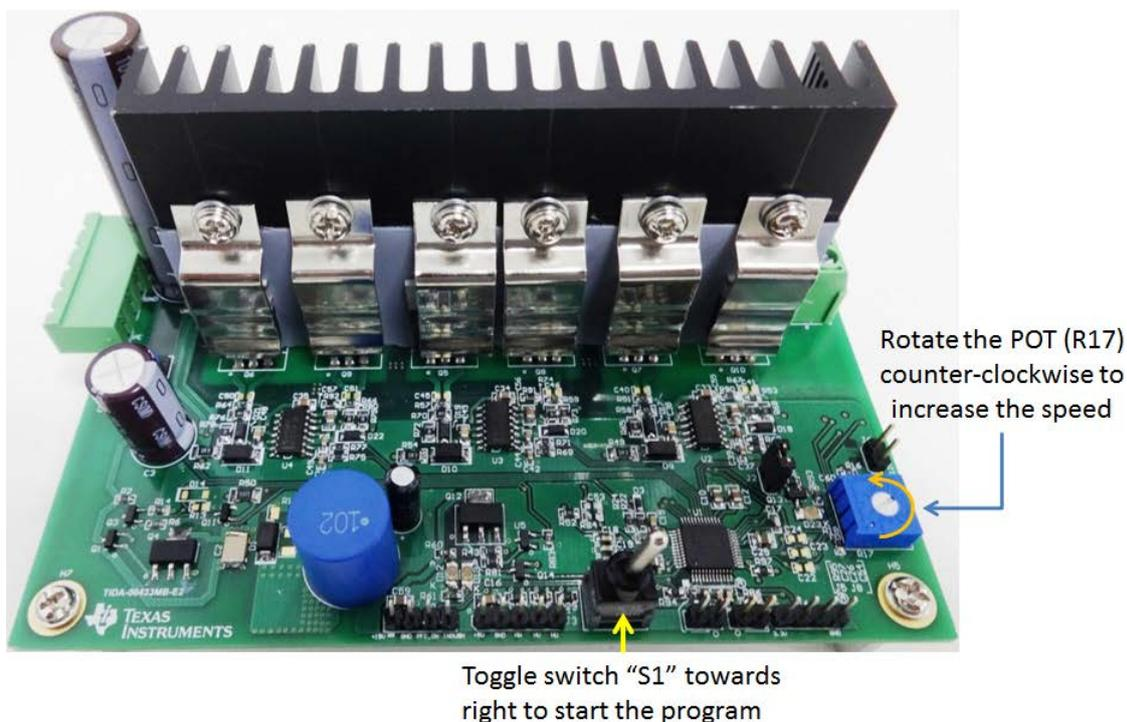
**Figure13. Program Start Up and Speed Variation Control**
