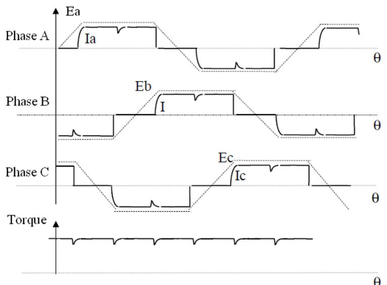
Fig 2. Electrical Waveforms in Two-Phase ON Operation and Torque Ripple
