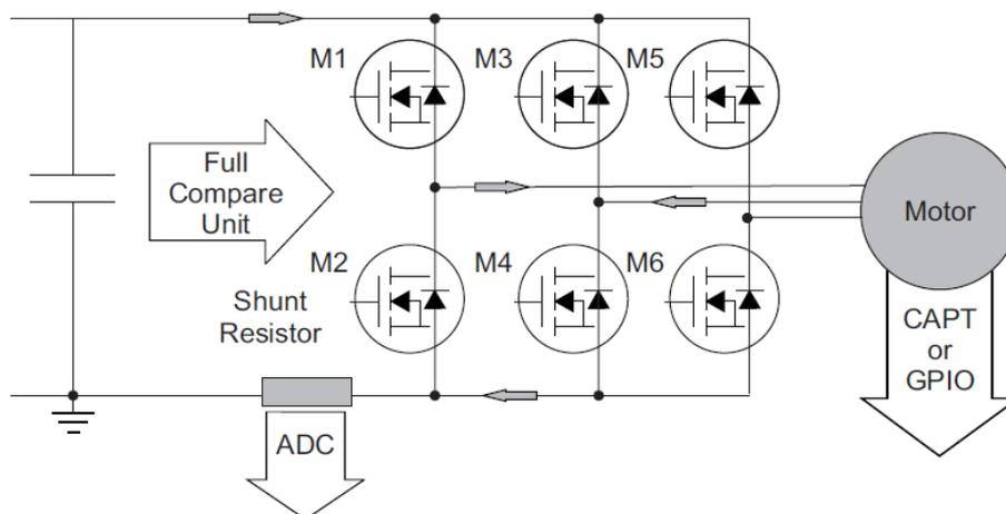
Fig.4 Three-Phase Inverter
