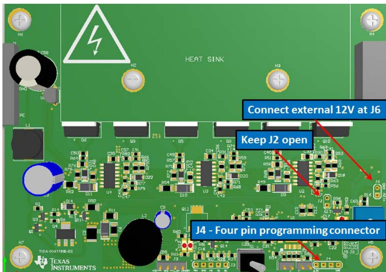
Figure 11. External Power Supply for Programming
