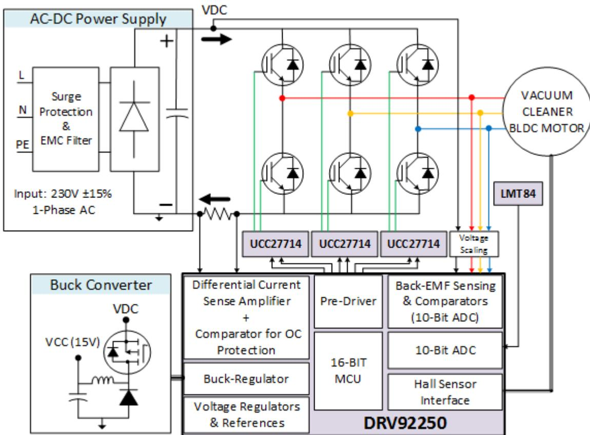
Figure 6. Overall Implementation of BLDC Motor Drive Using DRV92250
