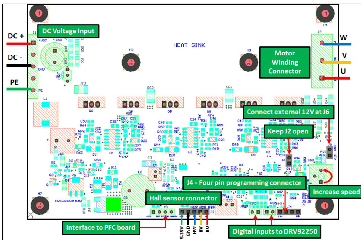
**Figure 13. System Interfaces and Connectors**
