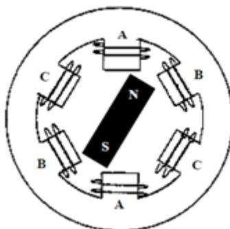
Fig 1. Three-Phase Synchronous Motor With One Permanent Magnet Pair Pole
