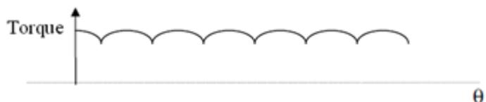
Fig.3 Torque Ripple in Sinusoidal Motor Controlled as BLDC
