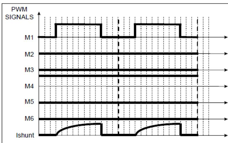
Fig. 5 Shunt Resistor Voltage Drop According to PWM Duty Cycles (Soft Chopping)
