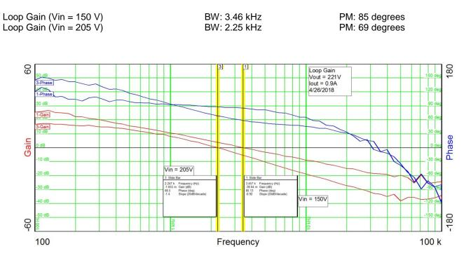
The plot below shows the boost converters loop gain with the input voltage set to 150 V and 205 V while loaded at 0.18 A.
