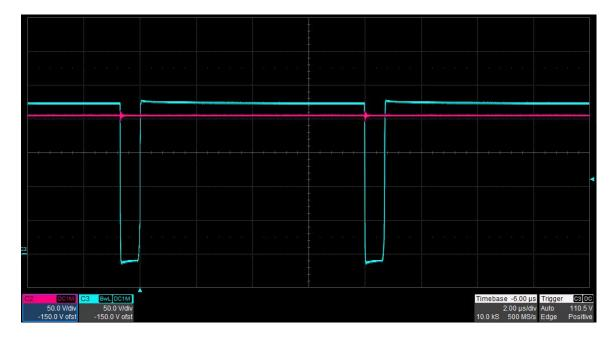
The photo below shows the FET switching voltage at TP2 and the input voltage. Vin = 205 V, Vout = 221 V, lout = 0.18 A. (50 V/DIV, 2 uS/DIV)
