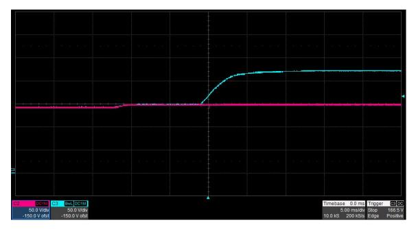
The photo below shows the startup of the 221 V output voltage (Blue) after the input voltage (RED) crosses the UVLO threshold of 142 V. lout = 0.9 A. (50 V/DIV, 5 mS/DIV)
