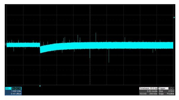
The photo below shows the 221 V output voltage (ac coupled) when the load current is stepped from 0.9 A to 0.45 A. Vin = 150 V. (1 V/DIV, 5 mS/DIV)
