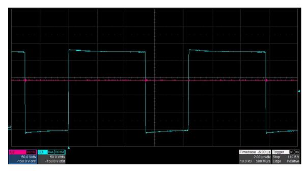
The photo below shows the FET switching voltage at TP2 and the input voltage. Vin = 142 V, Vout = 221 V, Iout = 0.019 A. (50 V/DIV, 2 uS/DIV)
