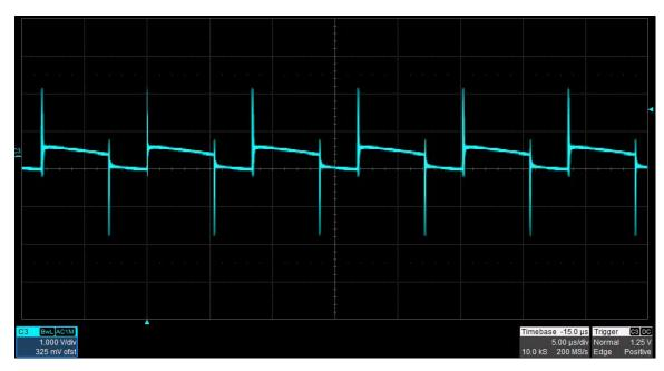
The output ripple voltage (AC coupled) is shown in the figure below. BWL = 20 MHz, Vin = 205 V, Vout = 221 V, Iout = 0.9 A (1 V/DIV, 5 uS/DIV)
