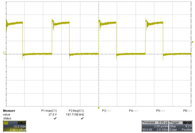
Figure 7. Primary Switching Node with 9 Vdc input
