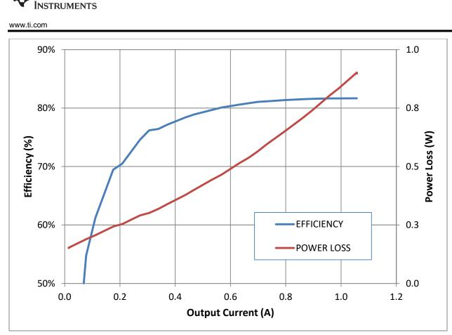
Figure 4. Efficiency with 15 Vdc input
