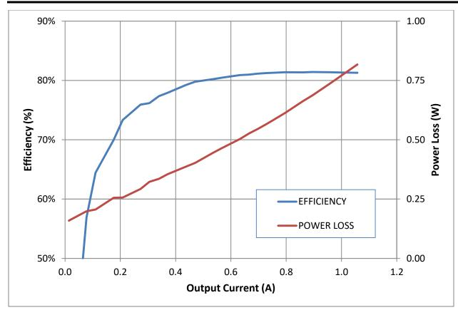
Figure 3. Efficiency with 12 Vdc Input
