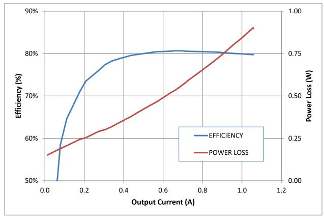
Figure 2. Efficiency with 9 Vdc Input
