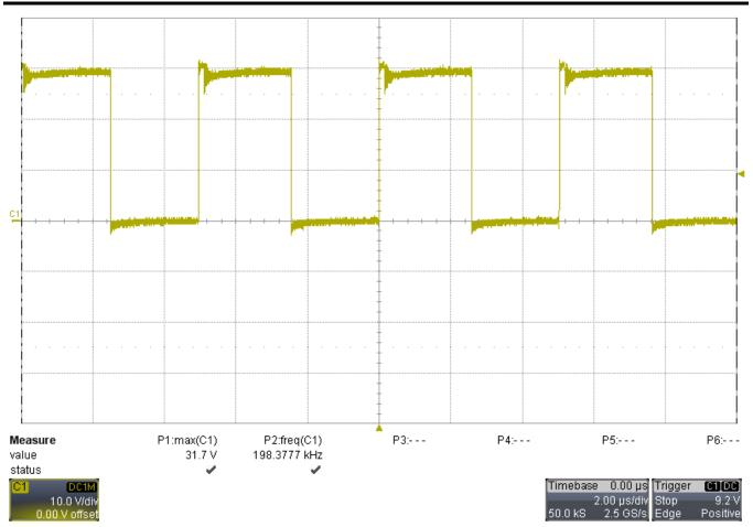
Figure 8. Primary Switching Node with 15 Vdc input
