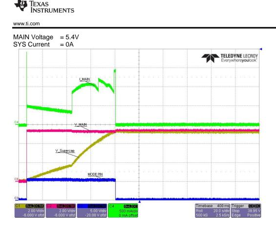
2.1.3 Supercap Charge; Input current limit Variant 2 (R7 = 130mohm, R5 = 0, R13 = R14 = R15 = DNP, R16=49.9ohm); Maximal charge current: 50mA , maximal precharge current = 50mA
