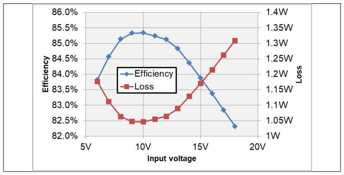
Figure 5 Efficiency and Loss vs Input Voltage
