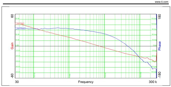
Figure 19 Bode Plot for 6 V Input Voltage
