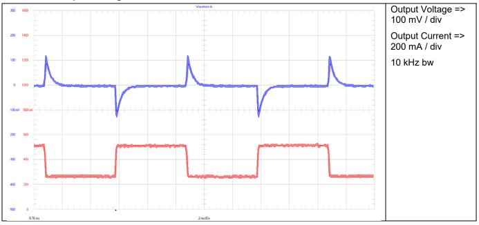
Figure 24 Load Transient @ 18 V Input Voltage
