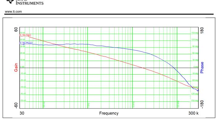
Figure 21 Bode Plot for 18 V Input Voltage
