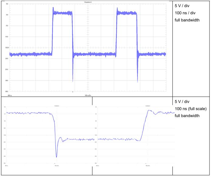
Figure 13 Waveform D2 to VOUT @ 6 Vin
