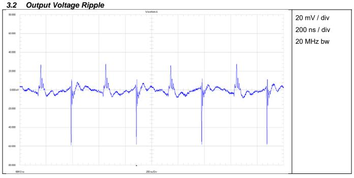
Figure 16 Output Ripple @ 12 V Input Voltage, output ripple 90mVpp, <1% Vout (!)
