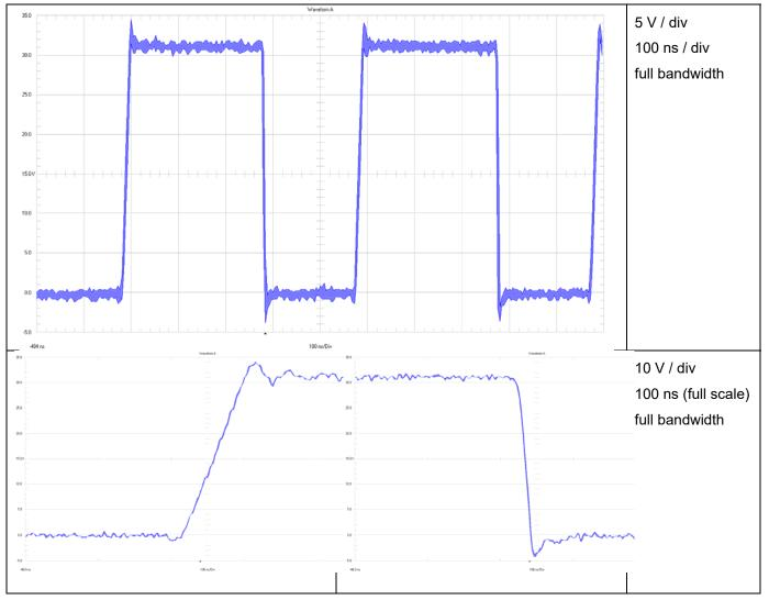
Figure 11 Waveform Q1 Drain to GND @ 18 Vin
