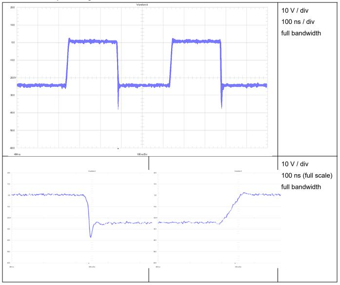
Figure 14 Waveform D2 to VOUT @ 12 Vin
