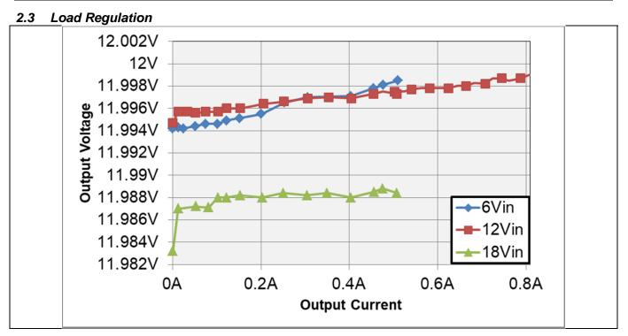
Figure 3 Output Voltage vs Output Current
