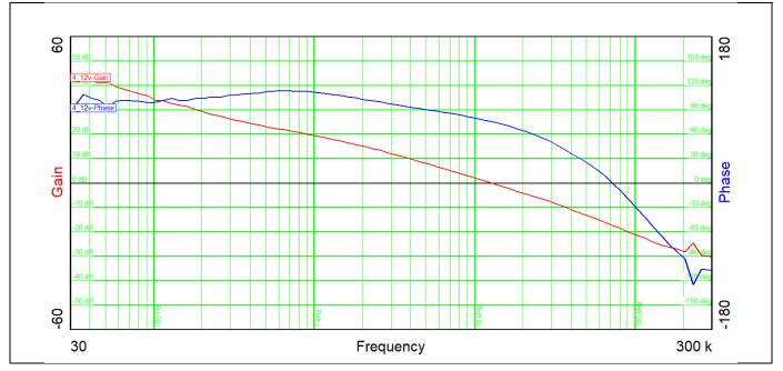
Figure 20 Bode Plot for 12 V Input Voltage
