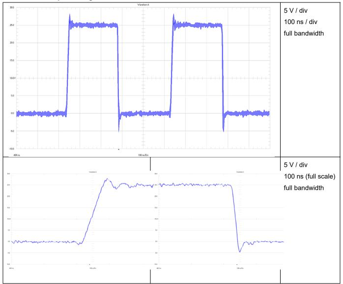
Figure 10 Waveform Q1 Drain to GND @ 12 Vin – almost neither overshoot nor ringing (!)
