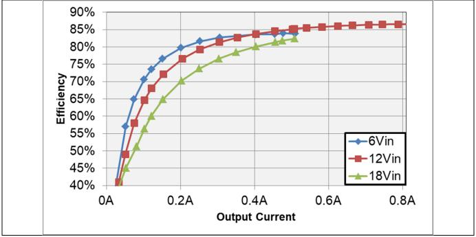
Figure 1 Efficiency vs Output Current
