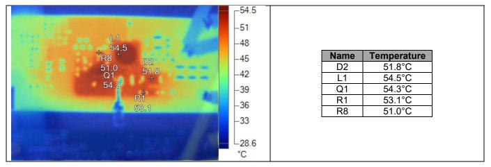
Figure 7 IR-Image @ 12 V Input Voltage – at nominal input dt < +35K (!)
