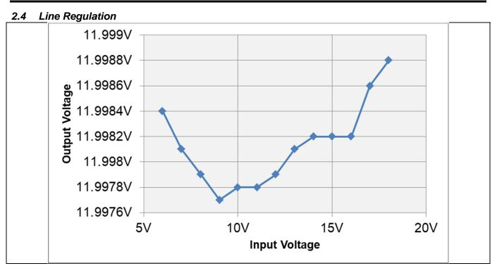
Figure 4 Output Voltage vs Input Voltage
