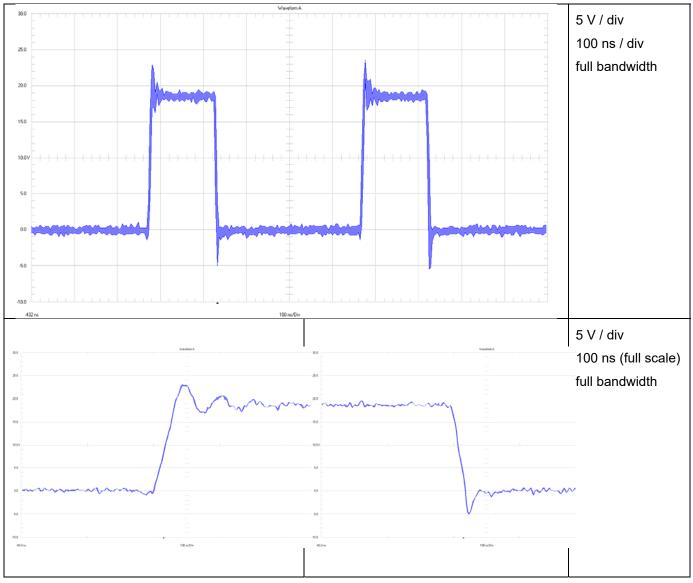
Figure 9 Waveform Q1 Drain to GND @ 6 Vin
