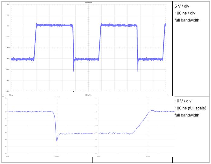
Figure 15 Waveform D2 to VOUT @ 18 Vin
