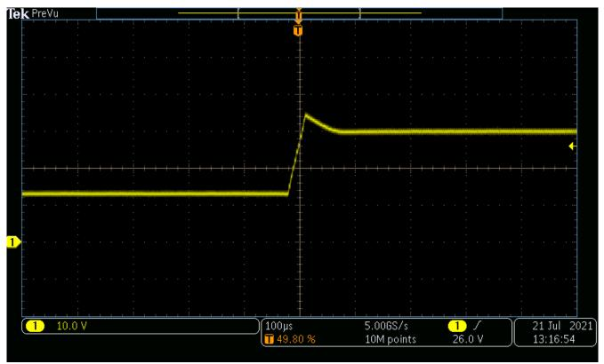
Figure 4-12. Boost Converter Start-up, 13.5 V<sub>IN</sub>, Maximum Load
