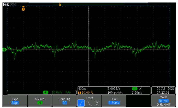
Figure 4-11. LLC Converter Output Ripple, 30  $V_{\text{IN}}$ , Maximum Load
