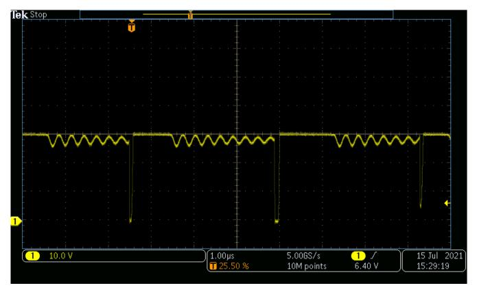
Figure 4-3. Boost Converter Switch Node, 28 V<sub>IN</sub>, Light Load
