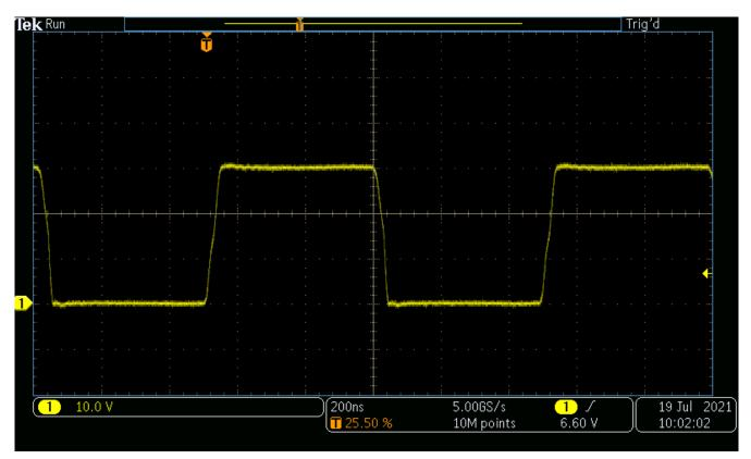
Figure 4-7. LLC Converter Primary Side Switch Node, 30  $V_{\text{IN}},$  Max Load
