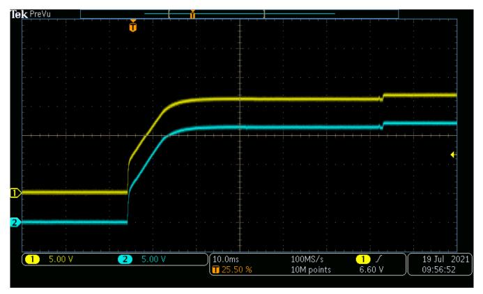
Figure 4-14. LLC Converter Start-up, 30 V<sub>IN</sub>, 50% Load
