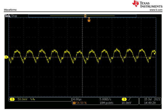
Figure 4-10. Boost Converter Output Ripple, 28 V<sub>IN</sub>, Maximum Load
