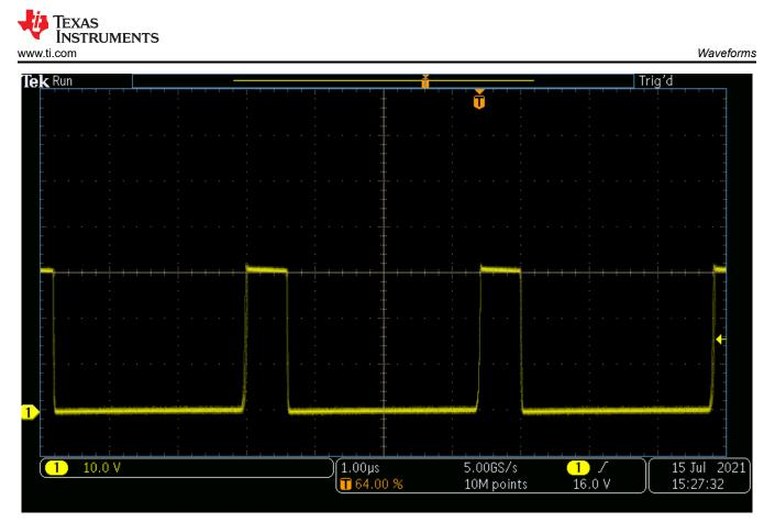
Figure 4-2. Boost Converter Switch Node, 6 VIN, Maximum Load
