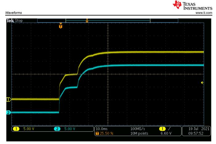
Figure 4-13. LLC Converter Start-up, 30 VIN, No Load
