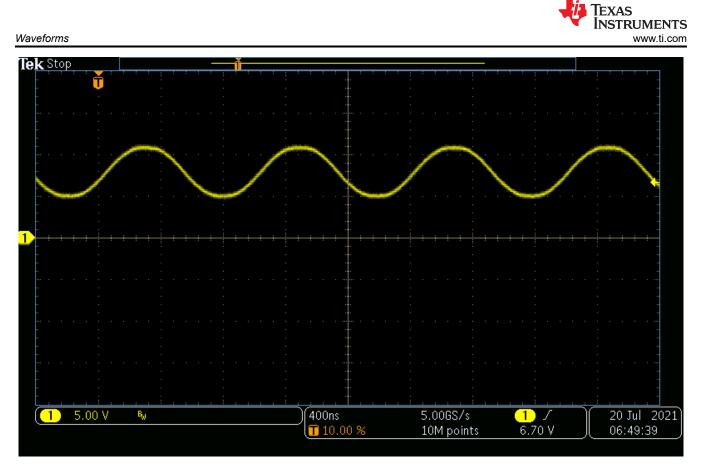
Figure 4-8. LLC Converter Secondary Side Resonant Capacitor, 30  $V_{\text{IN}},$  Max Load
