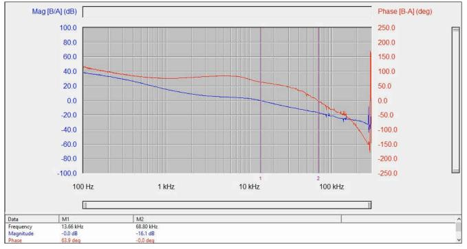
Figure 3-9. Loop Stability, 12  $V_{\text{IN}},$  250-mA Load
