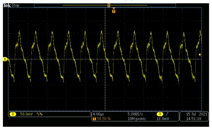
Figure 4-9. Boost Converter Output Ripple, 6 V<sub>IN</sub>, Maximum Load
