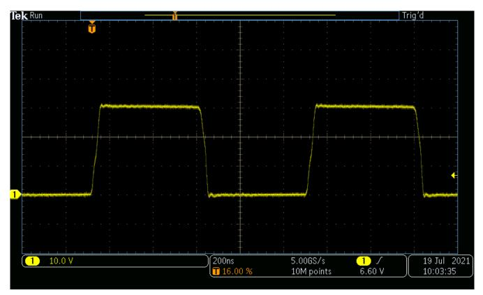
Figure 4-5. LLC Converter Primary Side Switch Node, 30  $V_{\text{IN}},$  No Load
