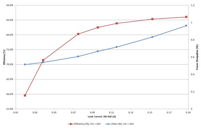
Figure 3-2. LLC Efficiency and Power Dissipation
