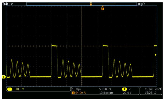
Figure 4-1. Boost Converter Switch Node, 6  $\rm V_{IN},$  Light Load
