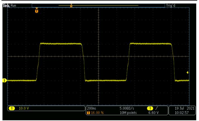
Figure 4-6. LLC Converter Primary Side Switch Node, 30  $V_{\text{IN}},$  50% Load
