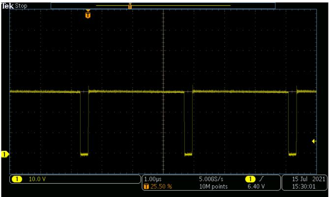
Figure 4-4. Boost Converter Switch Node, 28 V<sub>IN</sub>, Maximum Load
