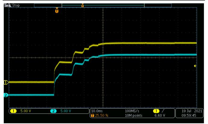
Figure 4-15. LLC Converter Start-up, 30 VIN, Maximum Load
