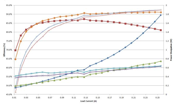
Figure 3-1. Boost Efficiency and Power Dissipation
