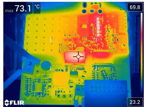
12 V<sub>IN</sub> to SEPIC, 24 V from SEPIC, +15 V, –5 V from isolated DC/DC. Isolated driver run at 40 kHz, 50% duty into 0.1- $\mu$ F load for 2  $\mu$ C per cycle or 80 mA, 1.6-W average current, power draw from isolated DC/DC. Ambient 21°C to 23°C with no fan. Isolated DC/DC at 73°C, gate driver at 56°C and gate drive resistors up to 76°C
