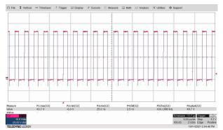
Figure 3-2. Switching at 18-V<sub>IN</sub> Q1 Drain Full Load at 445 kHz Showing 22 Cycles
