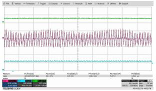
Figure 3-5. Output Voltage Ripple With 445-kHz Switching Frequency
