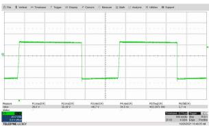
Figure 3-3. Switching at 42-V<sub>IN</sub> D1 Anode Full Load at 445 kHz Showing 2 Cycles
