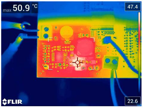
$V_{IN}$  = 18V,  $V_{OUT}$  = 24  $V_{OUT}$  at 130 mA The SEPIC switch is the hottest item.
