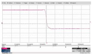
+15 V, -5 V to isolated driver, model t16 used Scope at full 500-MHz bandwidth
