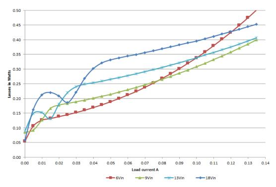
Figure 2-2. Power Loss of the PMP22817 SEPIC at 445 kHz
