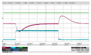
Green =  $V_{IN}$ , Pink =  $V_{OUT}$ , Blue = Load Current Figure 3-8. Load Transient,  $V_{IN}$  = 13 V, Switching Frequency = 445 kHz
