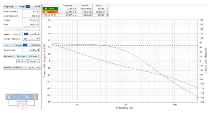
Figure 2-6. Bode Plot at 2-MHz Switching Frequency
