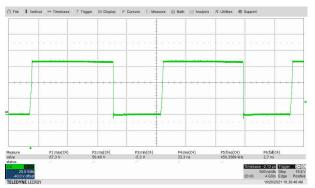
Figure 3-4. Switching 42-V<sub>IN</sub> Q1 Drain Full Load at 445 kHz Showing Two Cycles
