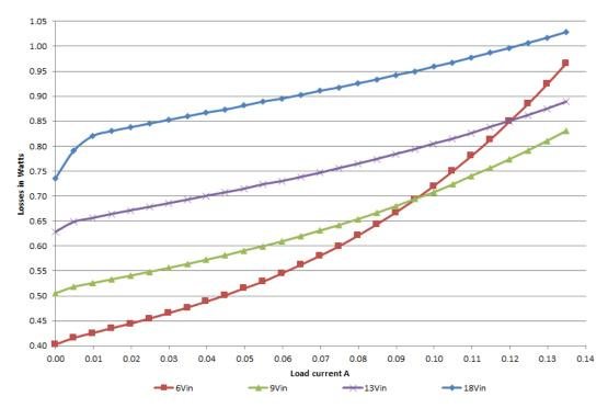
Figure 2-4. Power Loss of the PMP22817 SEPIC at 2 MHz
