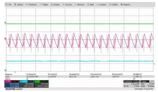
Figure 3-6. Output Voltage Ripple With 2-MHz Switching Frequency
