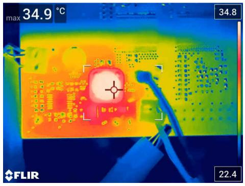
$V_{IN}$  = 18  $V_{IN}$ ,  $V_{OUT}$  = 24  $V_{OUT}$  at 130 mA The SEPIC inductor is the hottest item.
