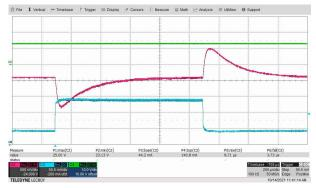
Green = V<sub>IN</sub>, Pink = V<sub>OUT</sub>, Blue = Load Current **Figure 3-9. Load Transient**, V<sub>IN</sub> = 13 V, Switching **Frequency = 2 MHz**
