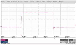
Figure 3-1. Switching at 18-V<sub>IN</sub> Q1 Drain Full Load at 445 kHz Showing Only 1 Pulse
