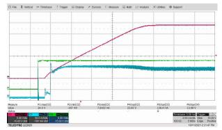
Green = V<sub>IN</sub>, Pink = V<sub>OUT</sub>, Blue = Load Current Figure 3-12. Start-Up, V<sub>IN</sub> = 13-V Load
