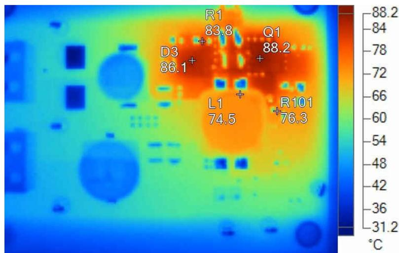
Figure 2-9. IR Photo With 2-A Maximum Output Current
