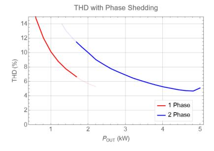
$V_{IN}$  = 230  $V_{RMS}$  $V_{OUT}$  = 400 V
