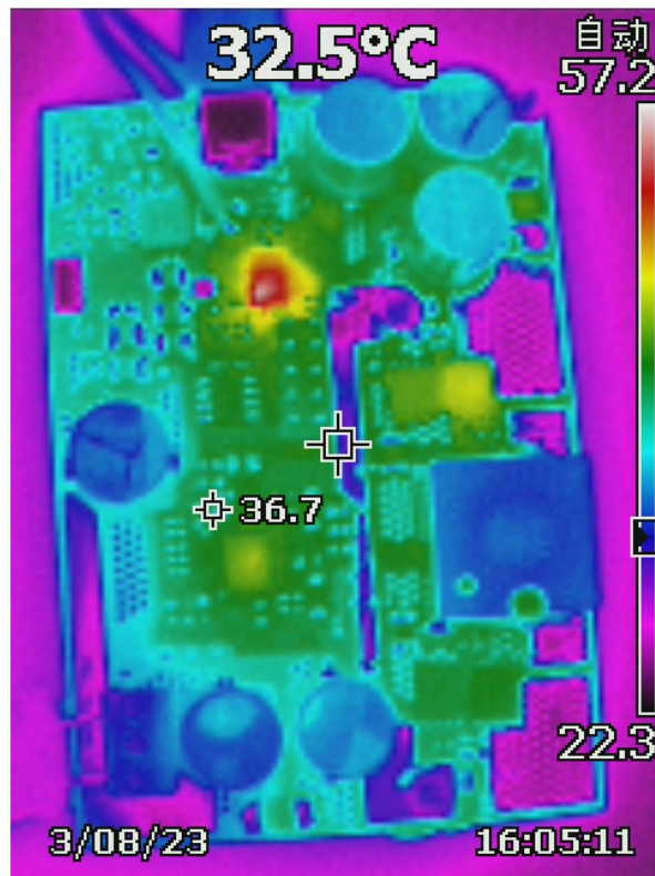
Figure 2-5. Charge Mode Thermal 20 Vsys to 4S Vbat
