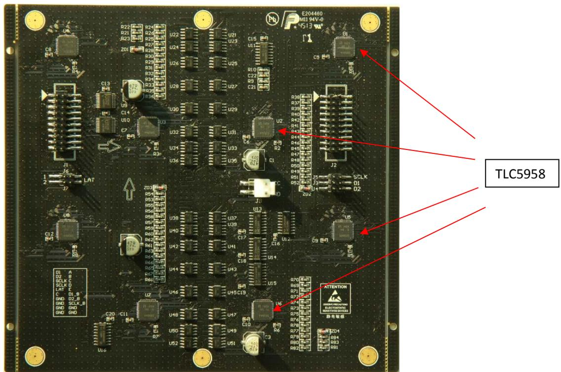
Fig2. Bottom view of LED module
