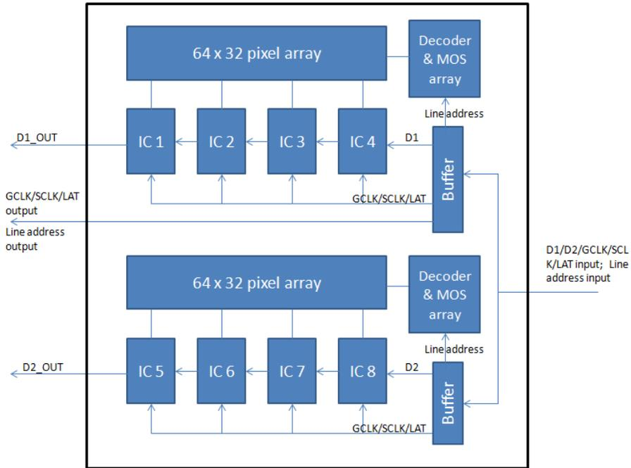
The whole module is divided into two parts, each include 64x32 pixel size, driven by 4pcs TLC5958 in series. Each 4pcs TLC5958 group have one GS data input port.
