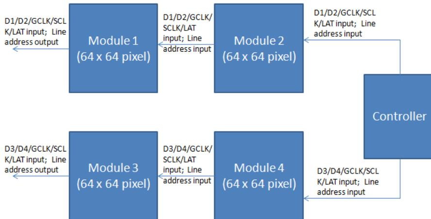
Module 1 and 2 are cascaded, use two GS data input ports D1 and D2. Same case for module 3 and 4. Because the total GS data transferred during one frame period is doubled, the minimum SCLK frequency should also be doubled.
