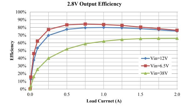
Figure 6 2.8V Output Efficiency
