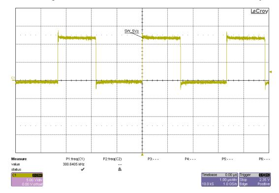
The switch node voltage waveform is measured at full load and no load condition for each output.
