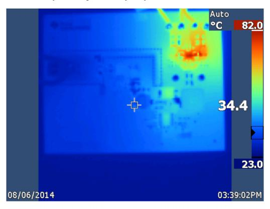
**Figure 3 Board Front Thermal Image**
