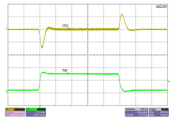
Figure 18 2.8V Output Buck Regulator Load Transient
