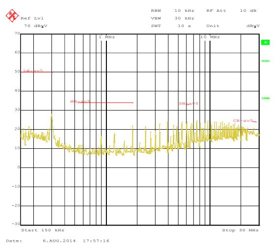
Figure 12 Peak detect, 150kHz – 30MHz
