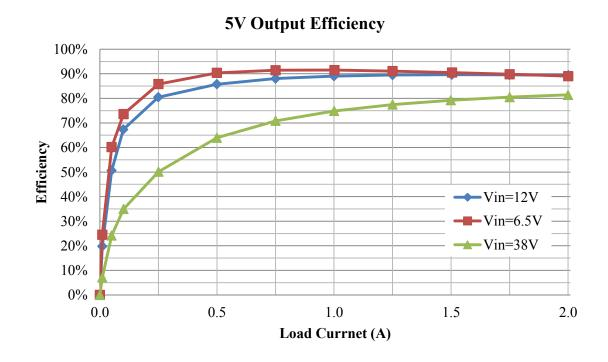
Figure 5 5V Output Efficiency
