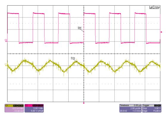
Figure 20 5V Output Ripple at 2A Load, 12Vin
