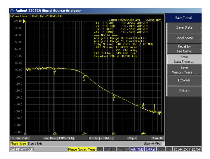
Figure 1. TRF3765 Output Phase Noise Plot
