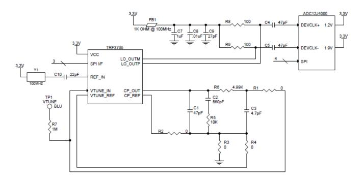
Figure 1. TRF3765 interface circuit to ADC12J4000
