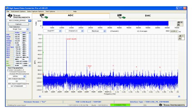
Figure 2. FFT performance of the ADC12J4000 with TRF3765 clock interface
