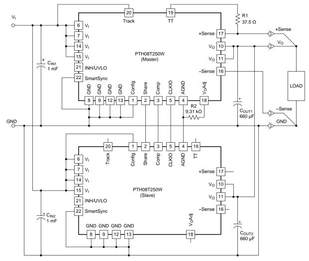
Figure 10. 100-A Current Source Design Schematic
