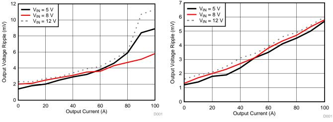
Figure 5. Output Voltage Ripple,  $V_{out}$  = 3.3 V
