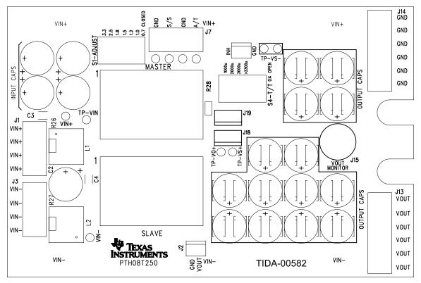
Figure 12. Top Layer (Top View)
