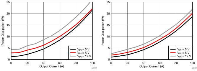
Figure 3. Power Dissipation, V<sub>out</sub> = 3.3 V
