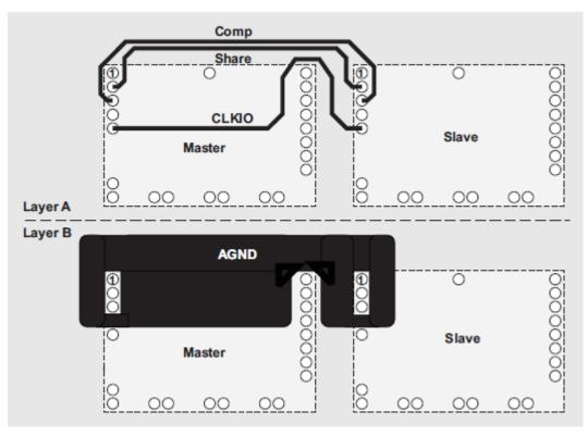
Figure 11. Board Layout Interconnection Pins
