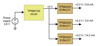
Figure 9. Test Setup — Buck Converter Output
