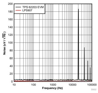
Figure 14. Noise Comparison at 3.3 V/3 mA
