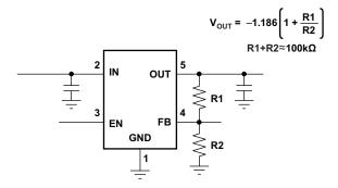
Figure 7. TPS72301 Typical Configuration
