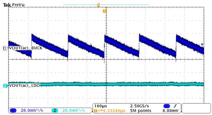
Figure 11. Ripple Comparison at 3.3 V/0.8 mA
