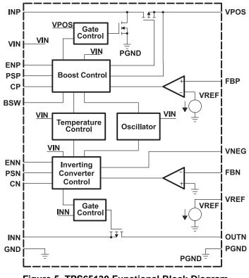
Figure 5. TPS65130 Functional Block Diagram
