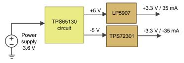
Figure 10. Test Setup — LDO Output
