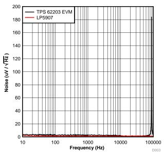
Figure 16. Noise Comparison at 3.3 V/14.2 mA
