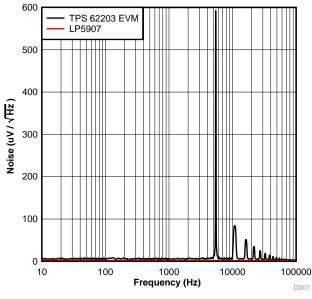
Figure 12. Noise Comparison at 3.3 V/0.8 mA
