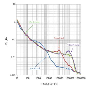
Figure 3. LP5907 Noise Density Test
