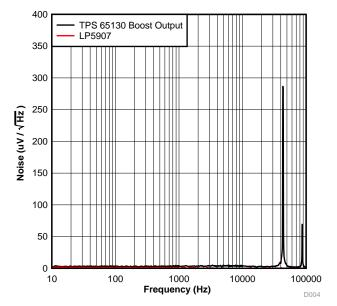
Figure 20. Noise Comparison Between LP5907 and TPS65130 Boost Output
