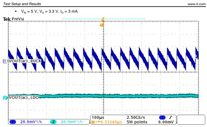
Figure 13. Ripple Comparison at 3.3 V/3 mA
