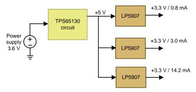
Figure 18. LDO Output for Amplifier
