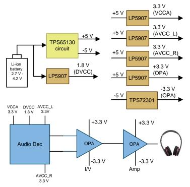
Figure 1. TIDA-00571 Block Diagram
