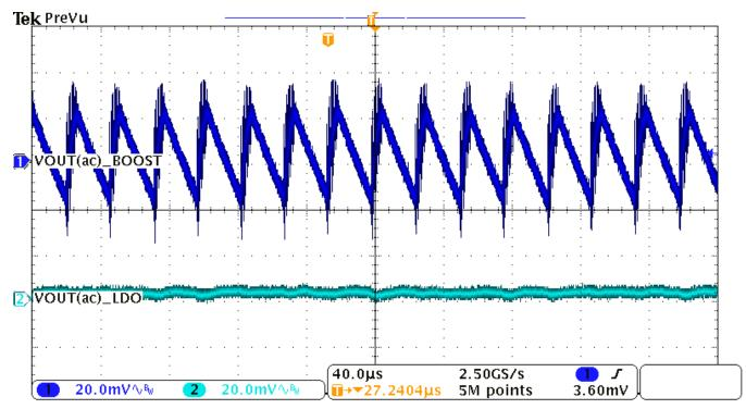
Figure 19. Ripple Comparison Between LP5907 and TPS65130 Boost Output
