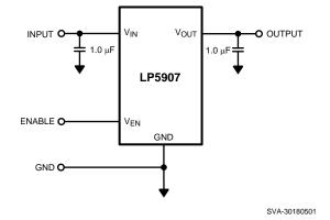
Figure 6. LP5907 Typical Application Circuit
