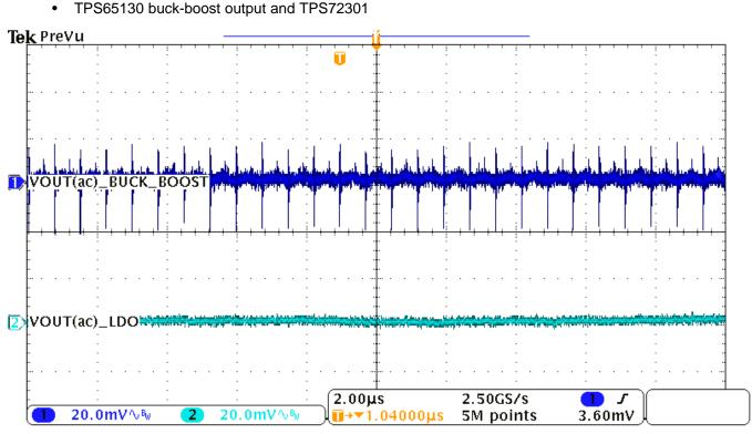
Figure 21. Ripple Comparison Between TPS72301 and TPS65130 Buck-Boost Output
