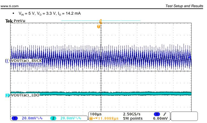
Figure 15. Ripple Comparison at 3.3 V/14.2 mA
