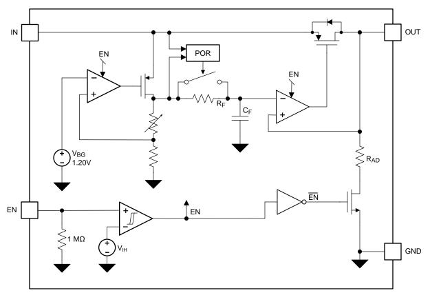
Figure 2. LP5907 Functional Block Diagram
