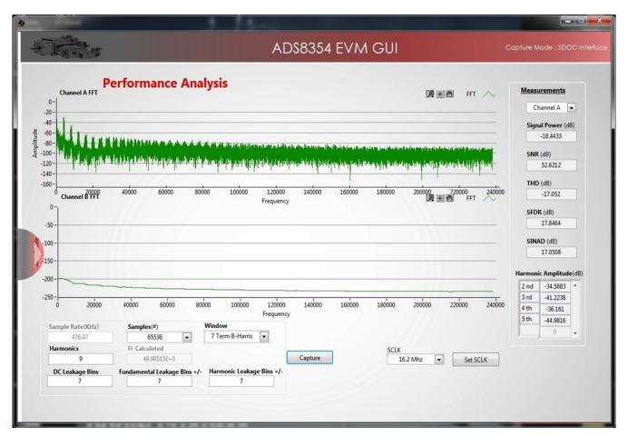
Figure 58. FFT of Motor Current (Measured Using ADS8354 EVM GUI)
