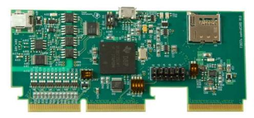
Figure 21. Image of Delfino™ F2837x Control Card from TI
