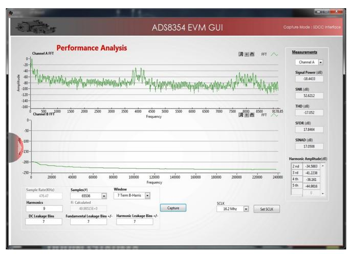
Figure 59. FFT of Motor Current (Zoomed-In) Showing Switching Frequency at 4 KHz and eHarmonics
