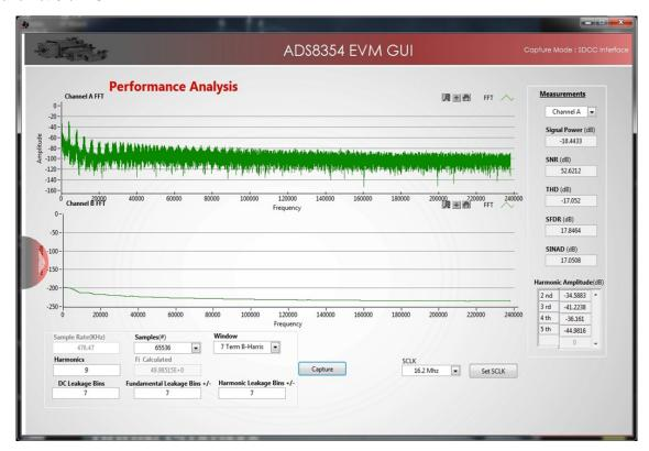
Figure 50. FFT Captured With ADS8354EVM GUI
