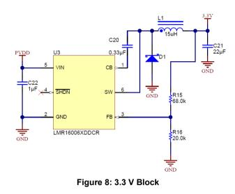
The LMR16006 is used as the basis for the 3.3 V supply. It is a regulated buck converter that takes the battery input voltage and steps it down to 3.3 V for the MCU. The input supply is bypassed with a 1  $\mu$ F ceramic capacitor and the output is filter with a 15  $\mu$ H power inductor and a 22  $\mu$ F ceramic capacitor. A feedback loop enables the converter to regulate to 3.3 V.
