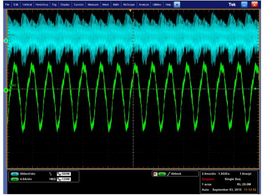
Supply voltage ripple at 80% speed command (6160 RPM).
