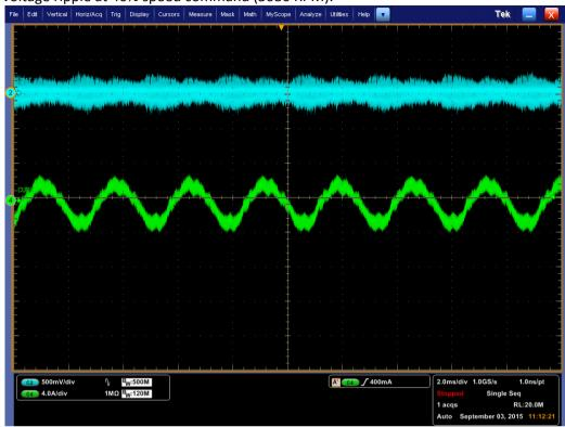
Supply voltage ripple at 40% speed command (3080 RPM).
