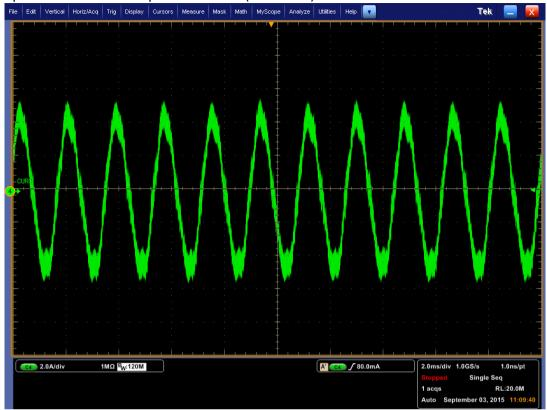
Motor phase current at 60% speed command (4620 RPM).
