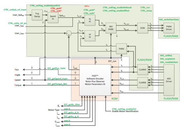
Figure 11: Software System Block Diagram
