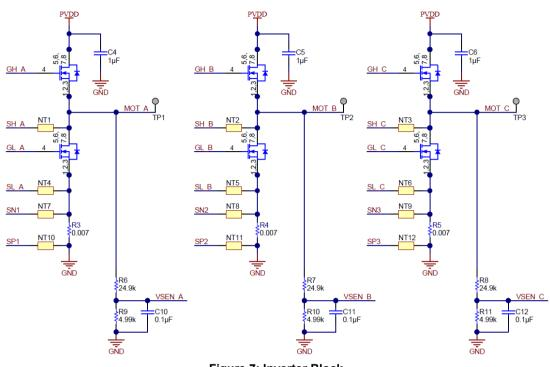
Figure 7: Inverter Block
