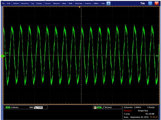
Motor phase current at 100% speed command (7700 RPM).
