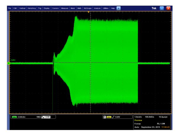
Test to examine motor ramping from stop (0 RPM) to full speed (7700 RPM).
