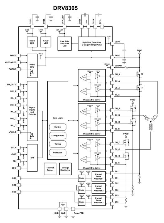
Figure 3: DRV8305 Block Diagram
