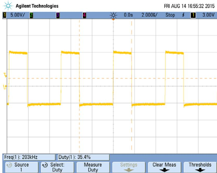
Figure 12 Switch node voltage at 10V input, full load
