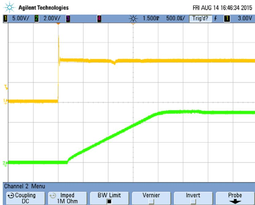
Figure 10 Power up into full load at 10V input
