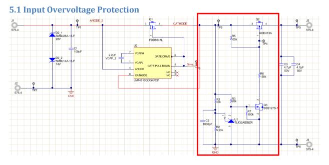
Discrete components are used for overvoltage protection. When the shunt regulator (U1) senses a voltage higher than 2.5V at R2, its output will go low which stops driving the N-channel FET (Q3). Q3 then acts as an open which ties the gate and source of the P-channel FET (Q2) together. The gate will not be driven which then prevents an output voltage. A timing capacitor (C2) is placed in parallel with R2 to prevent the circuit from outputting OV when there are quick high voltage surges.
