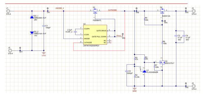
NOTE: TVS diodes are placed in both directions to protect the circuitry from high voltage transients.
