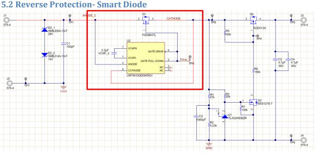
The LM74610 Smart Diode is placed before the overvoltage protection for reverse battery protection. For more information on the LM74610 functional and electrical characteristics, see the LM74610 Smart Diode Controller data sheet (<u>LM74610</u>).
