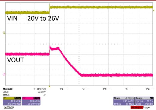
Transition to overvoltage condition. Protection at 25V.
