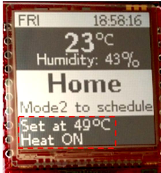
Figure 32. Messages Received on ETS to Turn On the Heater On and Turn Off the AC
