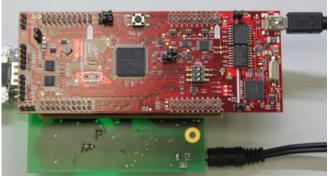
Figure 25. TIDA-00202 Board Mounted on the InstaSPIN-MOTION LaunchPad (Bottom View)
