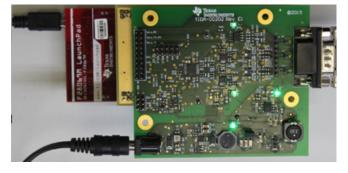
Figure 24. TIDA-00202 Board Mounted on the InstaSPIN-MOTION LaunchPad (Top View)
