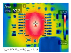
Figure 2. Input DCDC Converter Temperature Distribution
