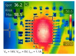
Figure 3. Input DCDC Converter Temperature Distribution
