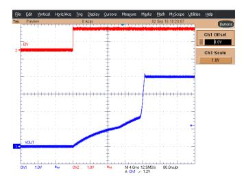
Figure 3. Startup With Resistor Load
