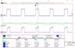
Figure 20. Current Sense Accuracy at 24% Duty Cycle
