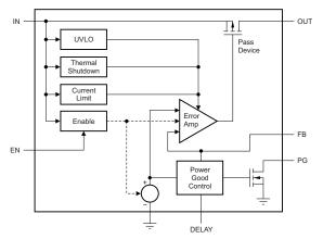
Figure 11. TPS7B8233-Q1 Functional Block Diagram
