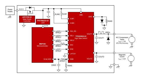
Figure 4. TIDA-00971 With LM74700-Q1 for Reverse Current Blocking
