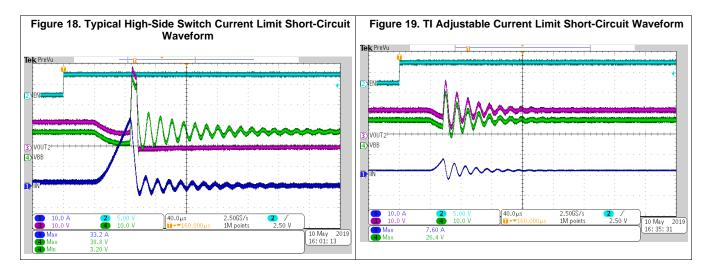
This is unacceptable for most applications that a short circuit on one output can cause other outputs to turn off. It is obvious that the cable inductance is causing the VBB of the device to ring which rings the output. However, with setting the current limit low for the specific load, the disturbance on VBB is limited and does not cause the entire part to go into an undervoltage event and shut down.
