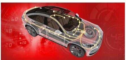
As Figure 5 illustrates, these wires can be up to 3 meters long and have to be routed around large mechanical components of the vehicle. This means that while the resistance is very low the inductance of the wire can be up to 5  $\mu$ H. This is also true of the output cables that go to the load. However, since they are obviously carrying less current than the input cable, their resistance per unit length will be high because they are smaller gage.
