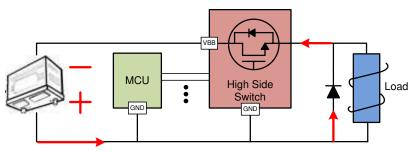
Figure 3. Reverse Battery Condition With a Shunting Diode Across Load
