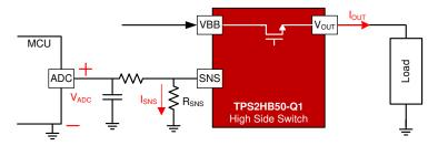
To calculate the total error in the system, several system tolerances must be accounted for.
