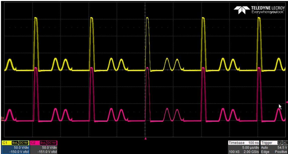
The photo below shows the FET switching voltage at TP4 (Red) and the voltage at D2-cathode (Yellow) for an output voltage of 150V, an input voltage of 15V and 0A load. (50V/DIV, 5uS/DIV)
