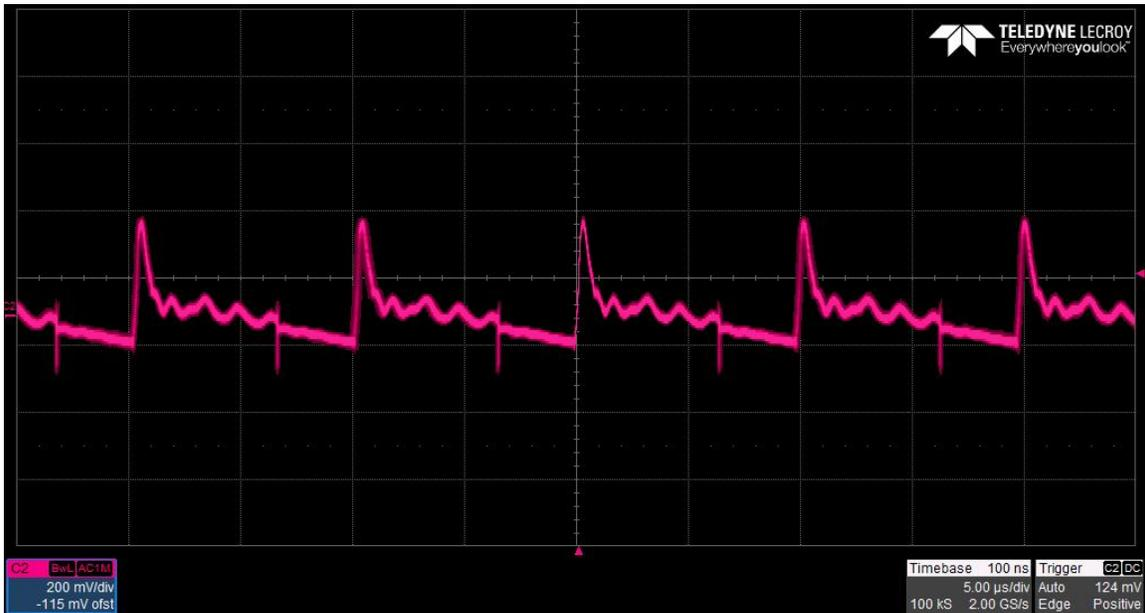
The 300V output ripple voltage (AC coupled) is shown in the figure below. The image was taken with the output loaded to 50uA. The input voltage is set to 9V. (200mV/DIV, 5uS/DIV)
