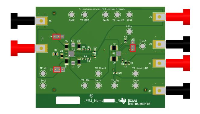
Figure 5. Power-Up Jumper Connections for Power Management Devices
