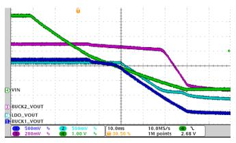
Figure 19. Shutdown Without Load
