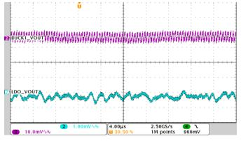
Figure 15. Buck 1 vs LDO Output Ripple
