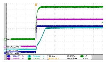
Figure 18. Start-Up Without Load
