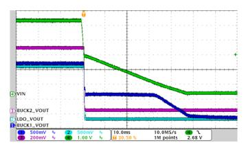
Figure 21. Shutdown With Full Load
