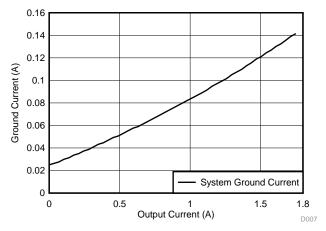
Figure 22. Active Mode Ground Current
