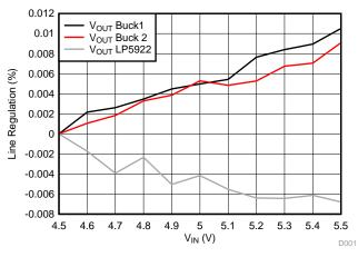
Figure 10. System Output Voltages Line Regulation
