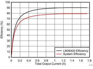
Figure 12. System Efficiency
