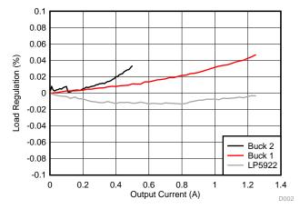
Figure 11. System Output Voltages Load Regulation
