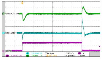
Figure 14. Load Transient Response
