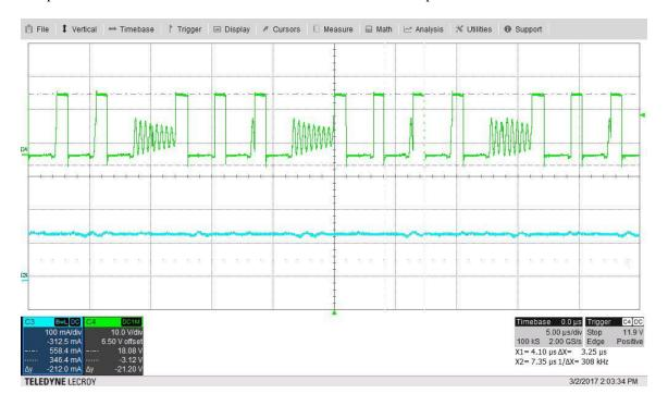
The photo below shows the switch node waveform with the -5.0V output loaded to 2A
