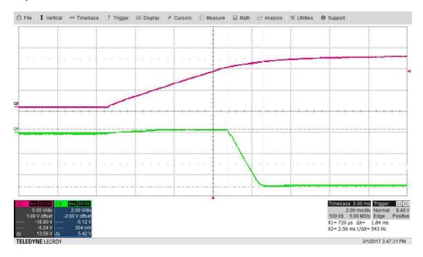
The photo below shows the output voltage startup waveform after the application of 12.0V in with the output loaded to -5.0V at 1A.
