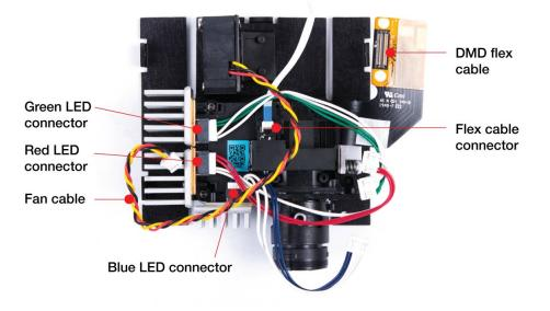
Figure 3-5. DLPDLCR230NPEVM Optical Engine Connection
