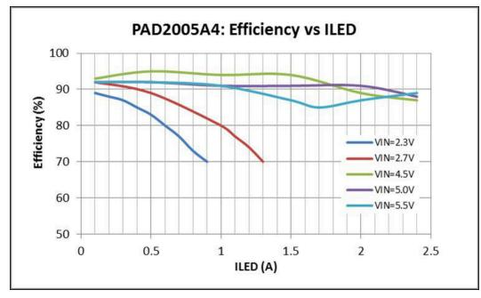
Figure 2-5. Measured Typical Power Converter Efficiency as a Function of ILED for Several Supply Voltages (V<sub>OUTmax</sub> = 4.8 V for Each Supply)
