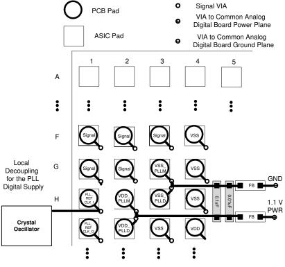
Figure 2-2. PLL Filter Layout
