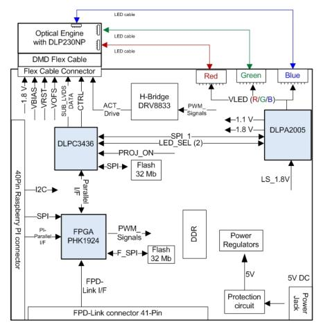
Figure 2-1. DLP LightCarfter Display 230NP EVM Block Diagram
