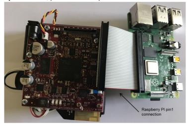
Figure 3-1. DLPDLCR230NPEVM With Raspberry PI
