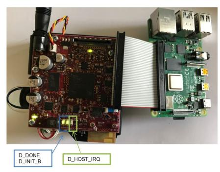
Figure 3-2. DLPDLCR230NPEVM LED Indications
