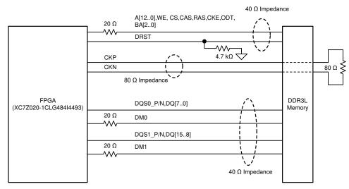
Figure 2-3. FPGA-DDR3L Interface
