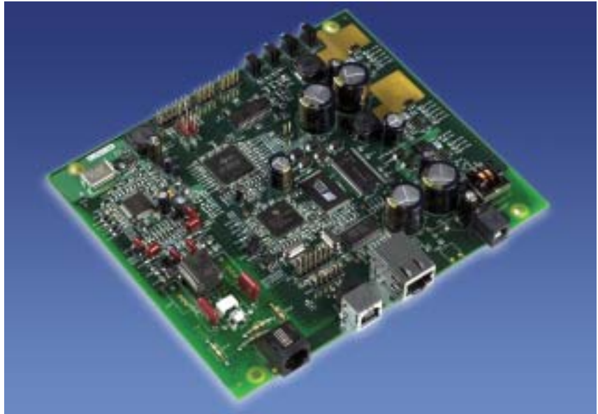
The AR5 platform for VoDSL offers up to eight channels of managed voice.
