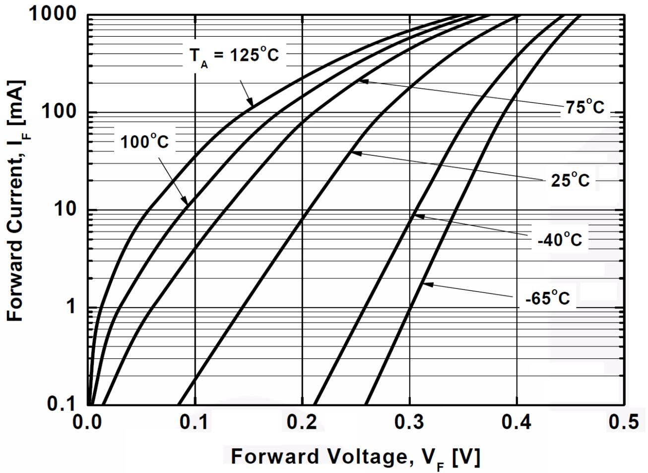
Figure 5-3. Forward Voltage of the Rectifier Diode
