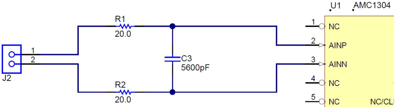
**Figure 3-1. AMC1304EVM Schematic: Analog Input Section**
