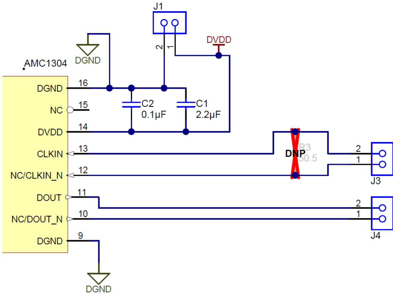
Figure 4-1. Power, Clock Input, and Digital Data Output
