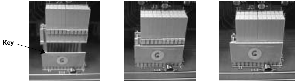
Figure 2–24. Connector Premate (Left), Mating (Center), and Mated (Right)
