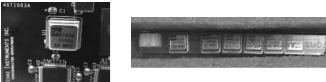
Figure 2–11. Clock Crystal on Card (Left) and Stored in Tube (Right)
