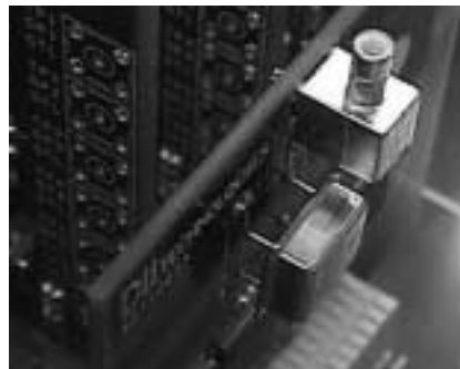
Figure 2–12. Clock Crystal With Leads in Position for Storage
