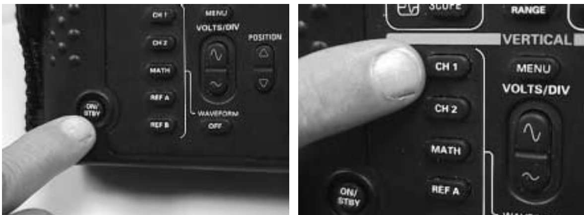
Figure 3–4. Turn On O-Scope (Left) and Select Channel (Right)
