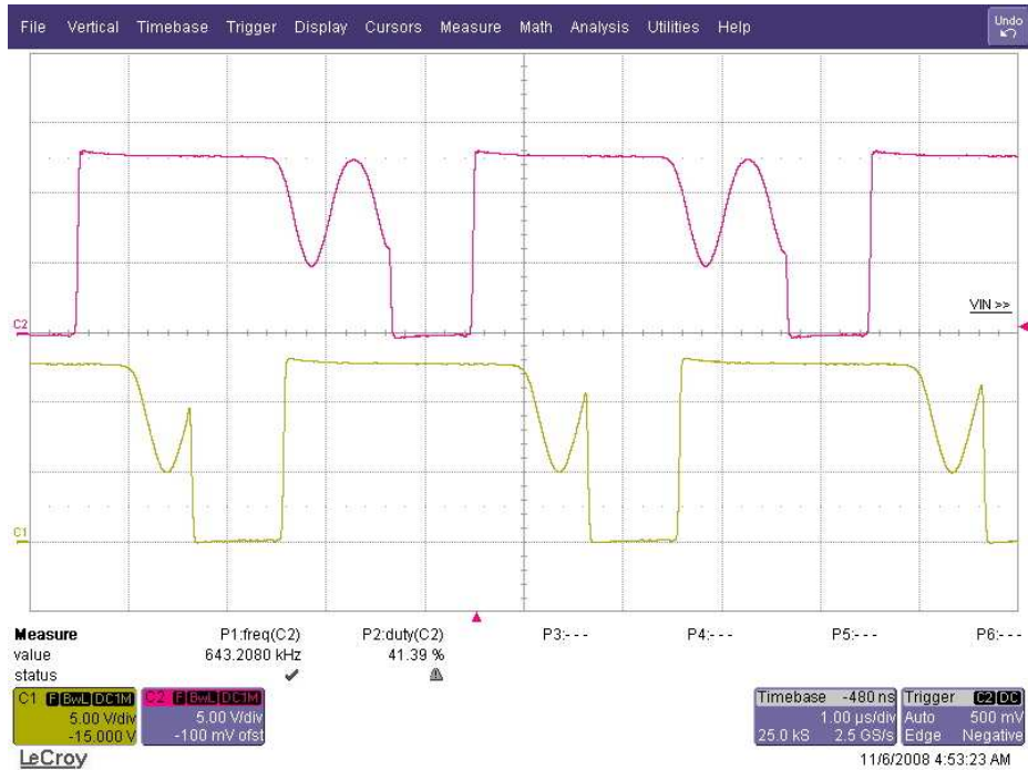
Current Sharing 1 (Iout<0.5A Vin=9V): VdsQ1, VdsQ2
