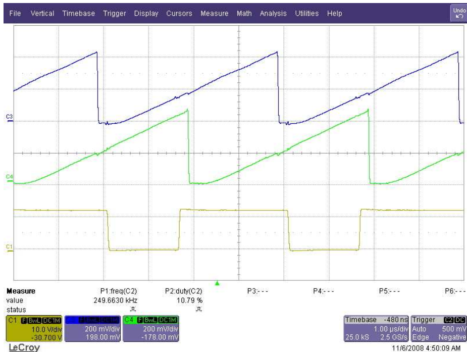
Synchronization Circuit 2: Out U3-TLC555D (C1), Synch_Master signal (C3), Synch Slave (C4)
