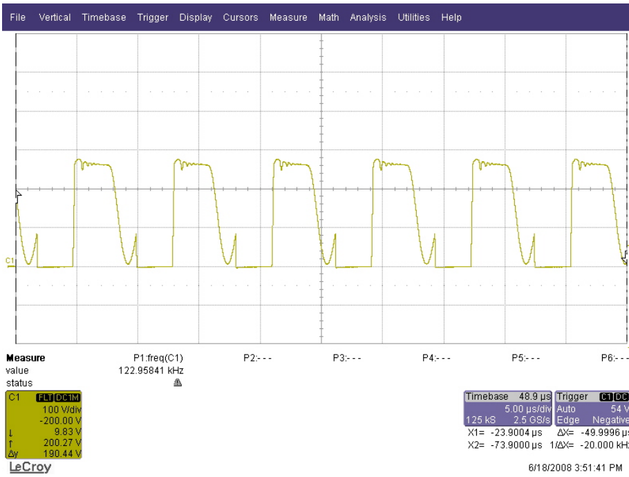
Primary Drain Voltage @ Vin peak=120V, 5V-50mA, 13.5V-100mA output
