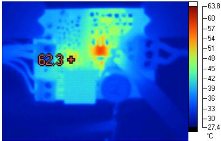
TOP Side Vin=375V peak, full Outputs Load
