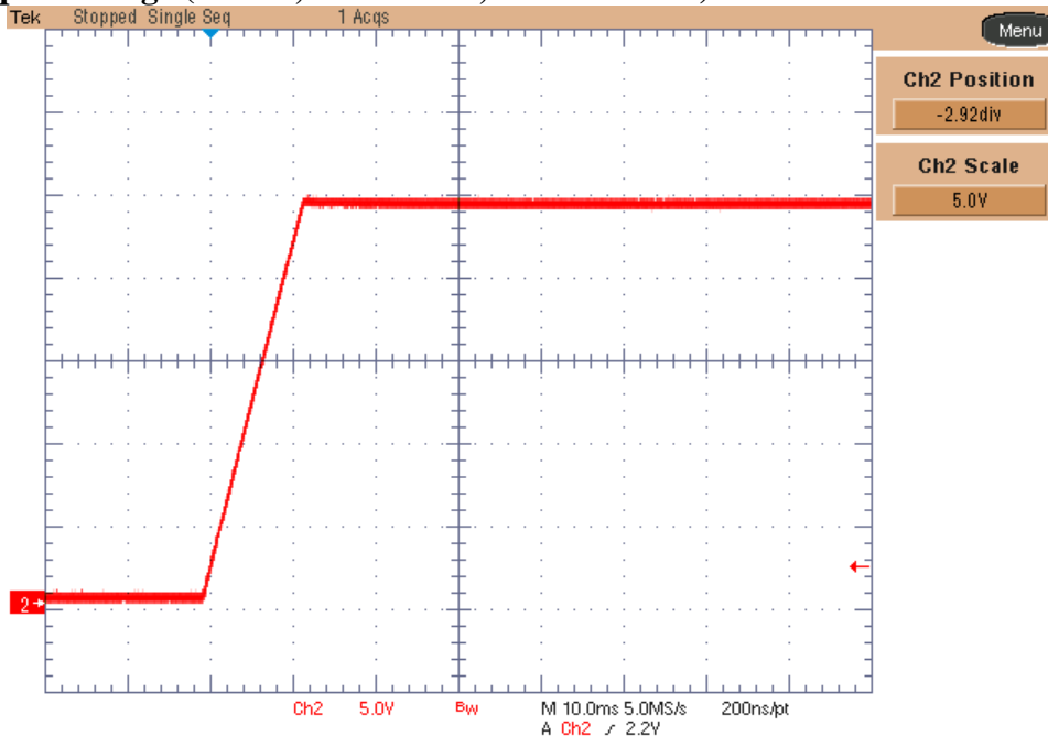
Ch.2: Output Voltage (5V/div, 10msec/div, 20MHz BWL) → No load
