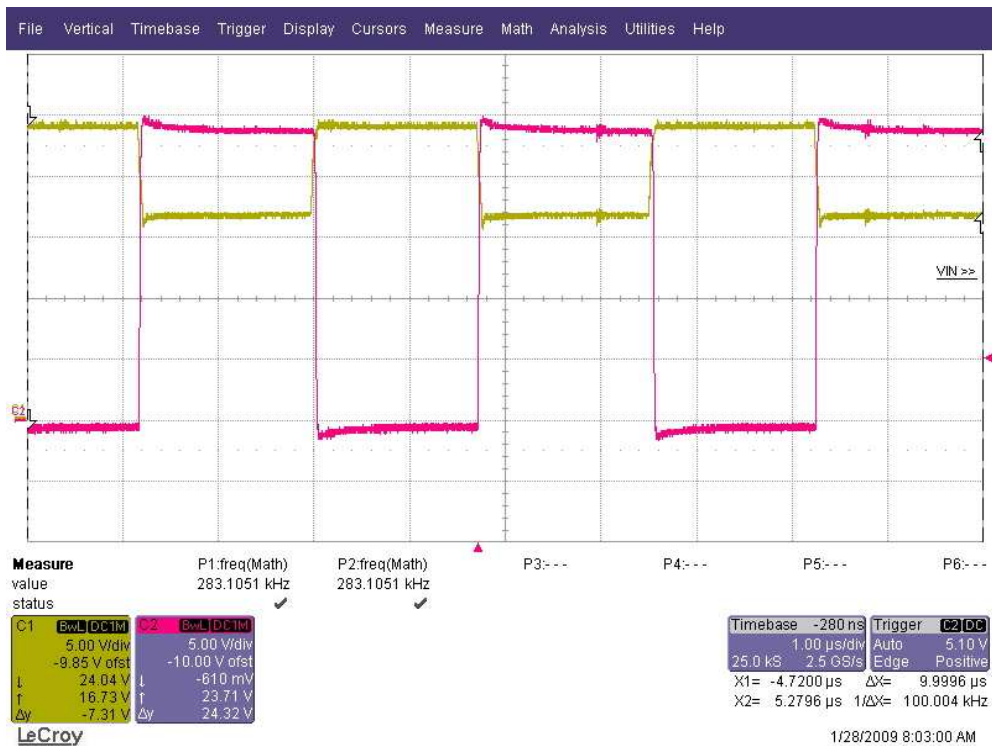
Switch Node and High Side Mosfet Gate of the 12V output Buck (TPS40200): VdGND Q4, TP26
