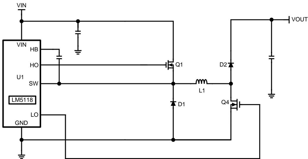
**Figure 1. Two Switch Simplified Block Diagram**
