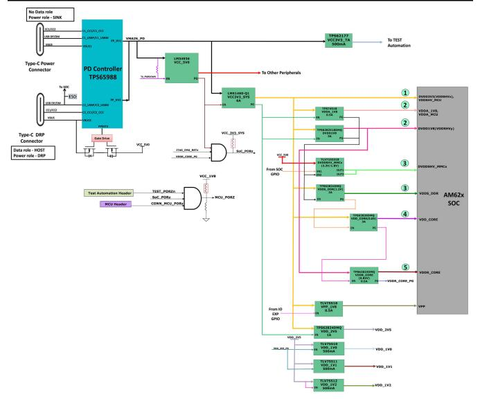
Figure 2-16. Power Sequence Block Diagram
