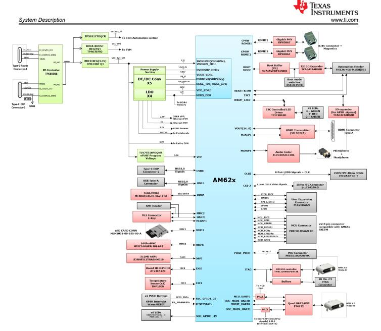
Figure 2-4. Functional Block Diagram of the SK-AM62B Board
