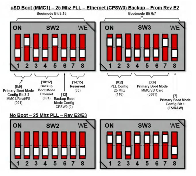
Figure 2-17. Bootmode Switch Configuration for SD Boot (From E2)
