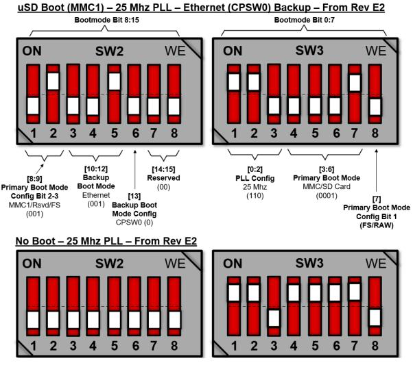
Figure 2-7. SD Bootmode Switch Setting Example (From E2)
