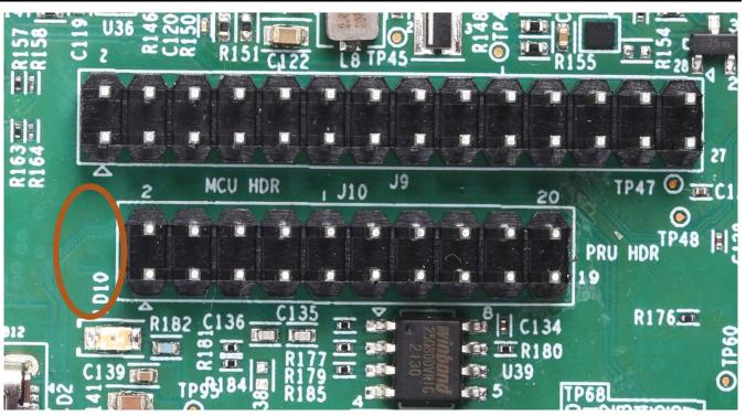
Figure 3-1. PRU Connector Missalignment on E1 Boards
