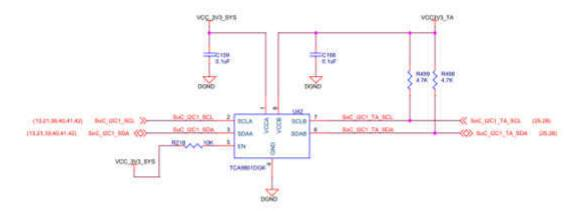
Figure 3-2. Schematic of I2C Buffer Section
