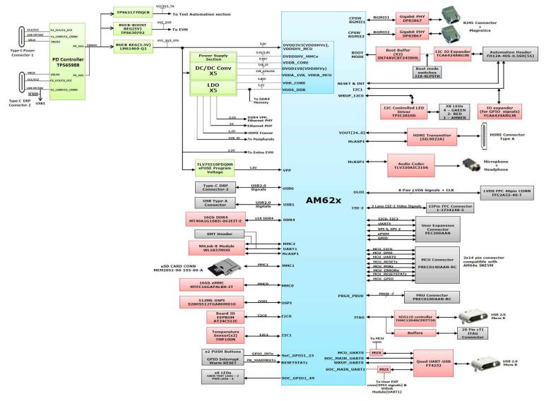
Figure 2-3. Functional Block Diagram of the SK-AM62 Board
