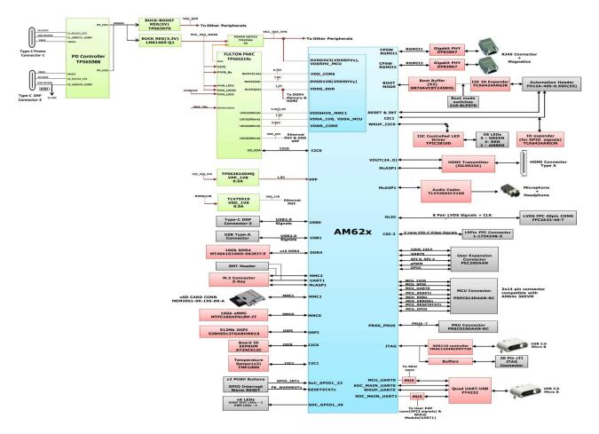
Figure 2-5. Functional Block Diagram of the SK-AM62-P1 Board with TPS65219 PMIC
