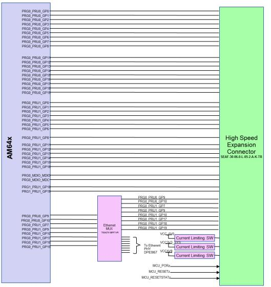
Figure 3-28. AM64x/AM243x High Speed Expansion Connector - Part 2
