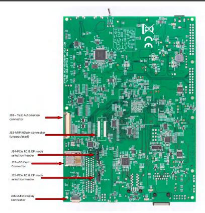
Figure 3-2. Bottom View of the AM64x/AM243x EVM Board
