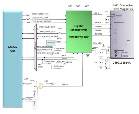
Figure 3-18. Ethernet Interface - CPSW Domain
