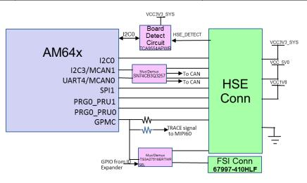
Figure 3-26. AM64x/AM243x High Speed Expansion Connector
