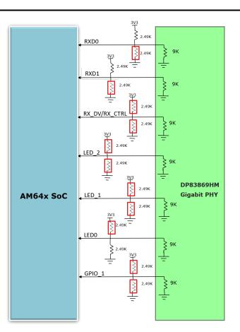
Figure 3-22. AM64x/AM243x Ethernet Interfaces - ICSSG2 Ethernet Strap Settings
