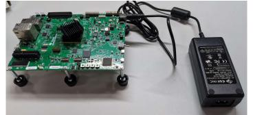
4. Apply AC power to AC/DC converter. 12 V power LED (LD6 and LD12) illuminates.
