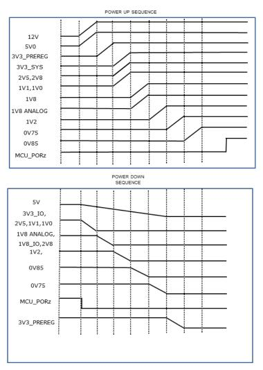
Figure 3-7. Power ON and OFF Sequencing
