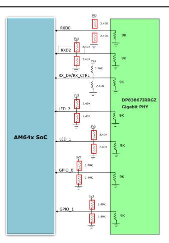
Figure 3-20. AM64x/AM243xEthernet Interfaces - CPSW Ethernet Strap Settings
