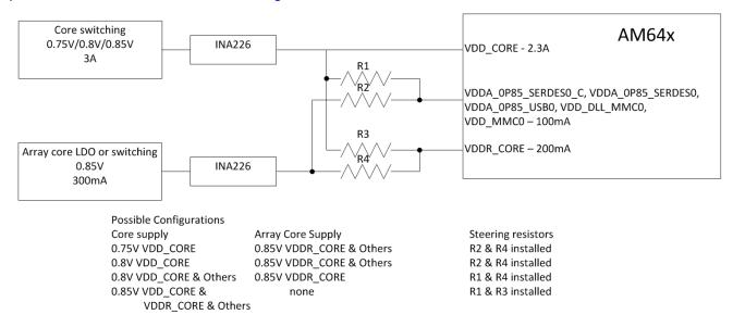
Figure 3-8. AM64x/AM243x Core Supply and Array Core Supply Options
