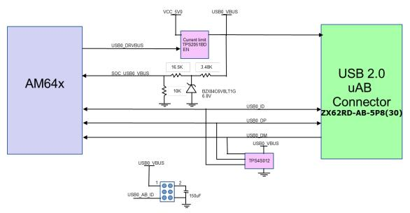
Figure 3-24. AM64x/AM243x USB 2.0 Host Interface
