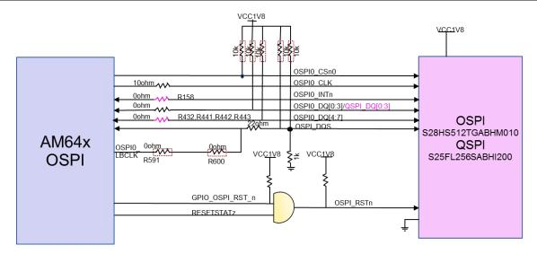
Figure 3-17. AM64x/AM243x OSPI Interface
