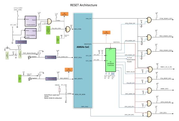
Figure 3-5. Overall Reset Architecture of the AM64x/AM243x EVM
