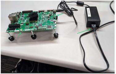
5. Place EVM power **(SW1)** switch in **ON** position as shown below.
