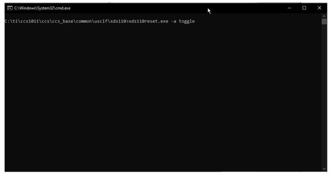
Figure 4-3. XDS110 debug reset utility command-line function
