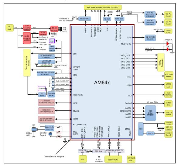
Figure 3-3. General Processor Board Functional Block Diagram
