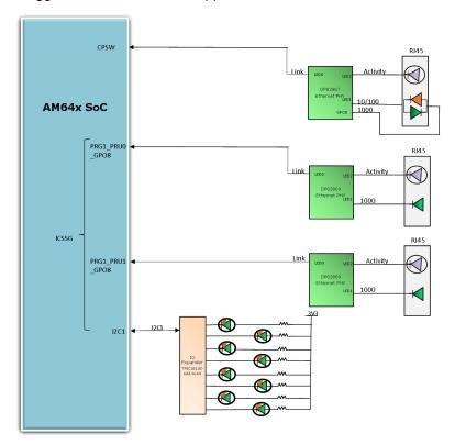
Figure 3-23. AM64x/AM243x EVM Ethernet Interface LED
