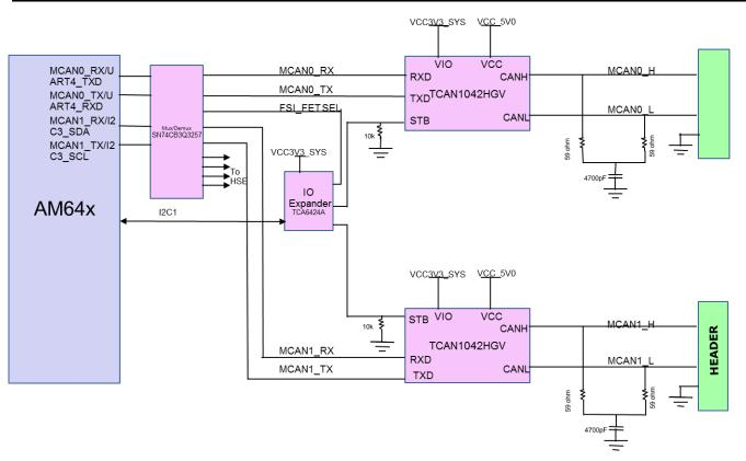
Figure 3-29. AM64x/AM243x CAN Interfaces
