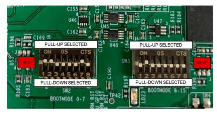
Figure 3-10. AM64x/AM243xEVM PCB, Boot Mode Selection Switches (SW2, SW3)
