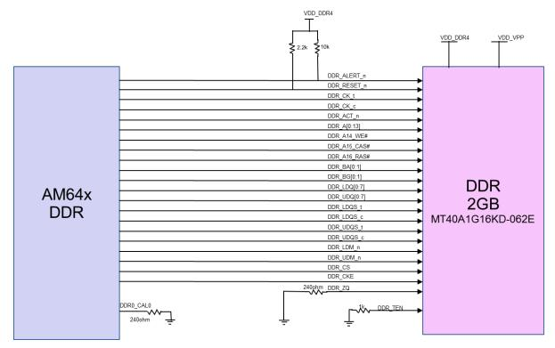
Figure 3-14. AM64x/AM243x DDR4 Interface
