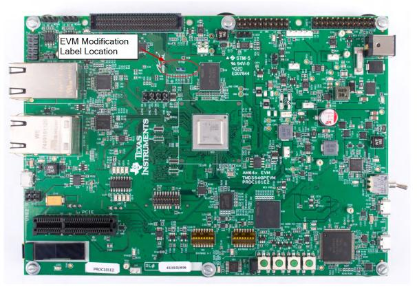
Figure 4-1. AM64x/AM243x EVM Modification Label Location
