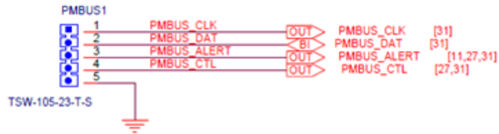
Figure 14. USB Pod to PMBus Header Connection
