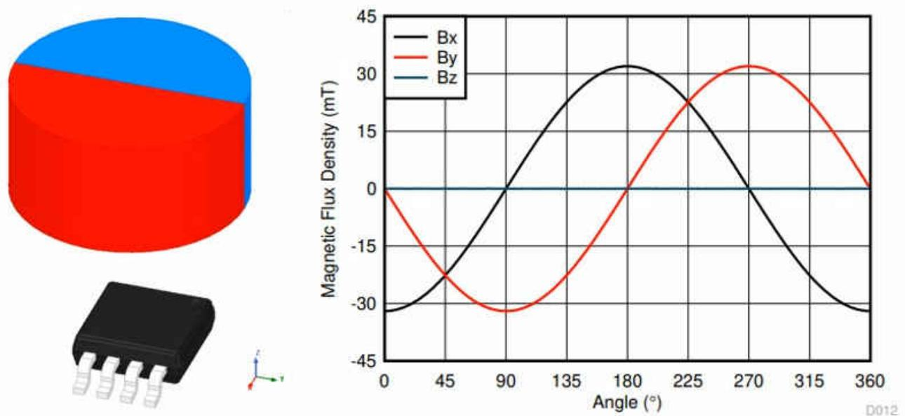
**Figure 2-5. 3D Linear Hall-Effect Sensor Magnet and Output Data**
