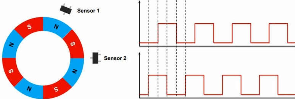
**Figure 2-4. Two-Sensor Implementation With Quadrature Output**
