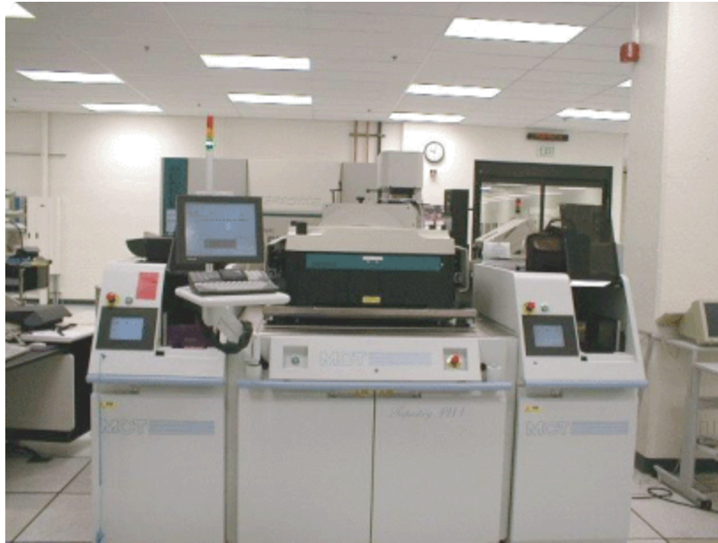
Figure 3 MCT Strip Test Handler with Teradyne A575
