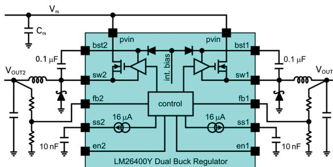
Figure 1. Simplified View of the LM26400Y Regulator
