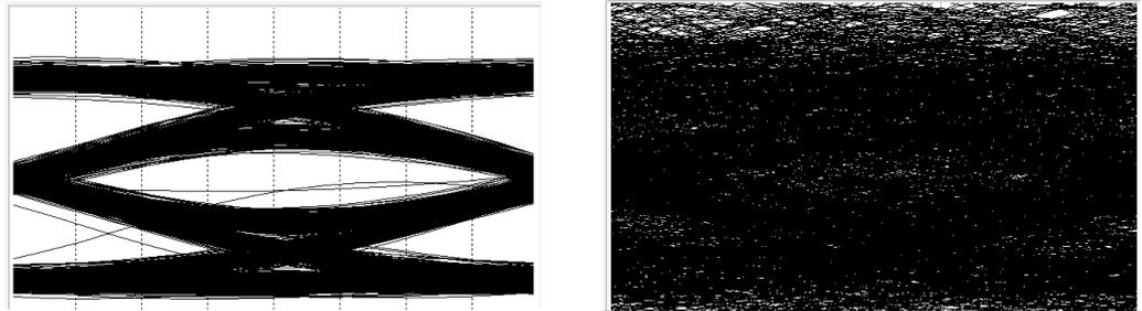
Figure 3 . Eye diagram uncoded vs. coded signal
